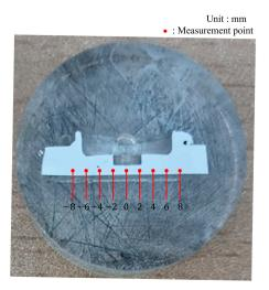
Figure 8. Measurement points for weld zone.
