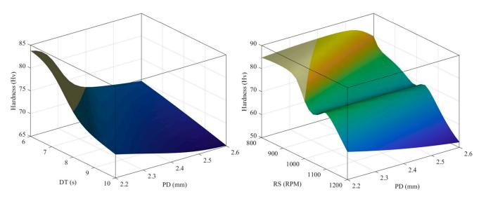
Figure 12. Predicted surface to hardness target based on design parameters.
