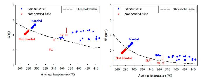
Figure 11. Results of bonding criterion according to threshold value.
