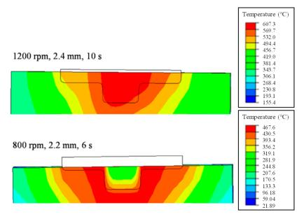
Figure 10. Typical cases of temperature distribution after the FSSW process.
