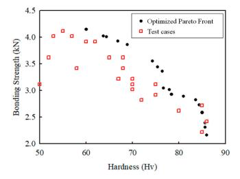
Figure 15. Results for the optimized Pareto front and all test cases.
