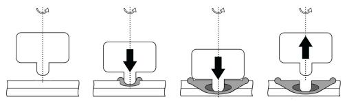
Figure 1. Schematic of the friction stir spot welding (FSSW) procedure.
