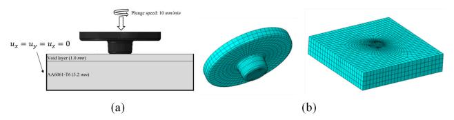
**Figure 6.** Schematic finite element (FE) model: (a) Boundary conditions of the FE model (b) Mesh of FE model.
