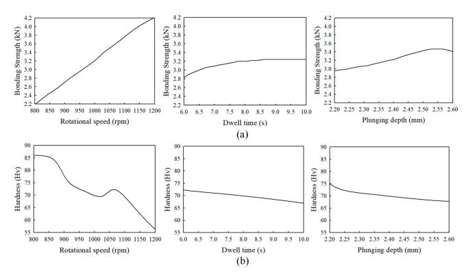
**Figure 14.** Variation of the objective functions (a) bonding strength and (b) hardness for each parameter when the other process parameters are held fixed.
