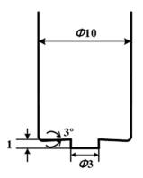
Figure 4. FSSW tool geometry.
