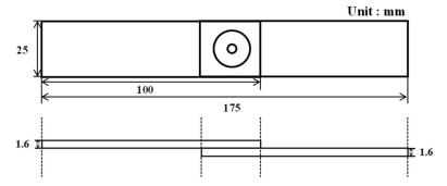
Figure 5. Typical specimen for lap-shear test.
