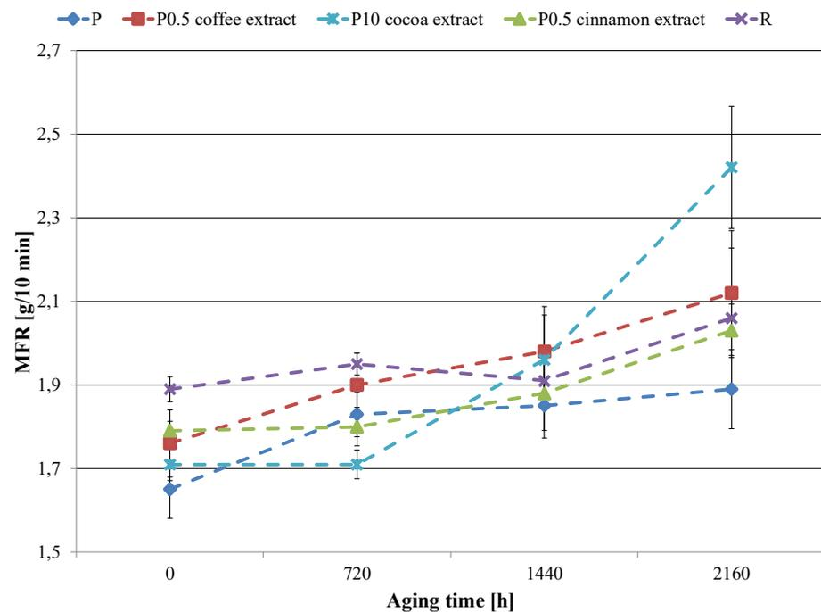
**Figure 3.** Melt flow rate (MFR) values of selected samples as a function of aging time.
