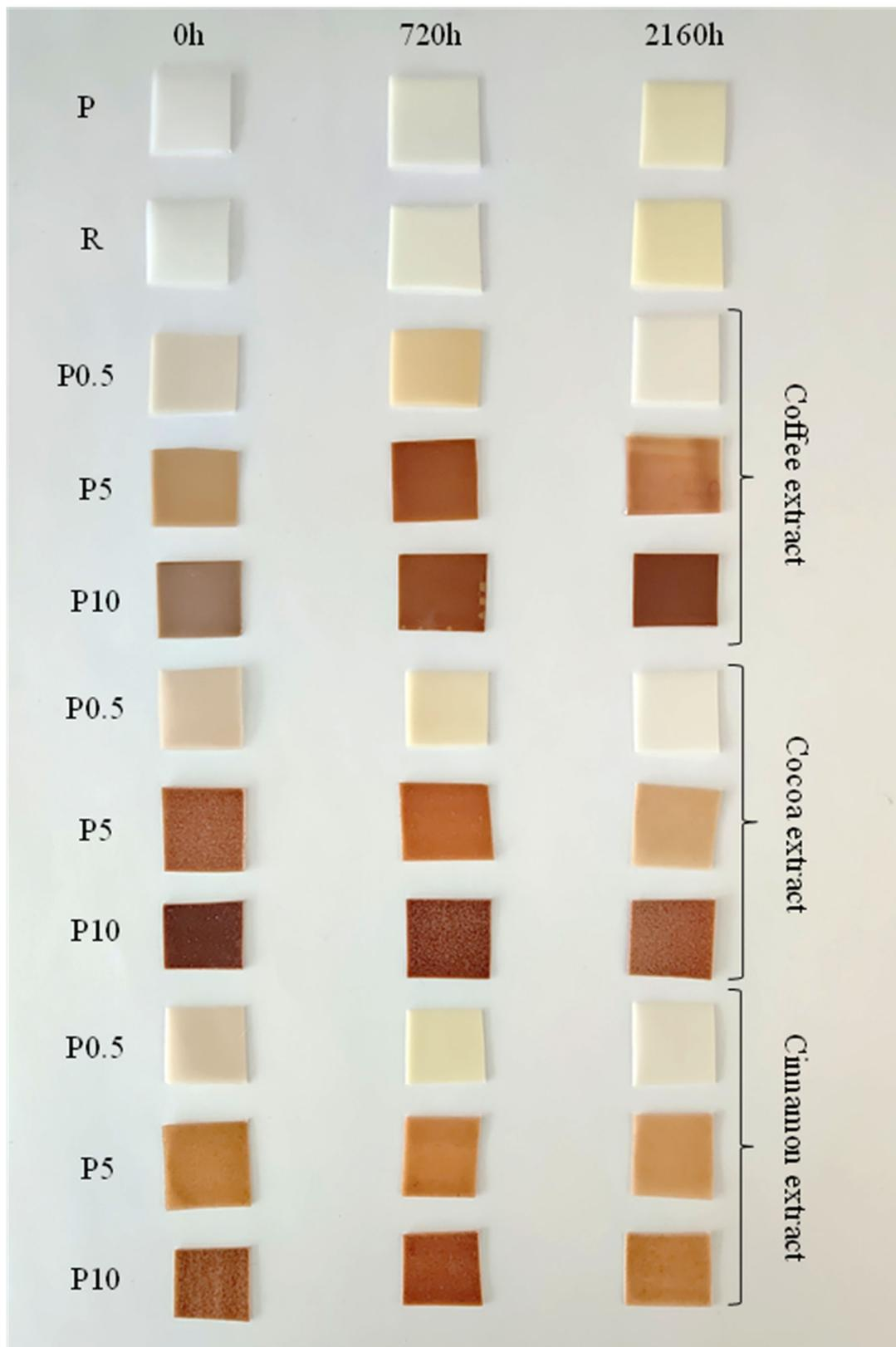
**Figure 1.** Photos of selected samples before and after the aging process. Approximate sample size 10 × 10 mm.
