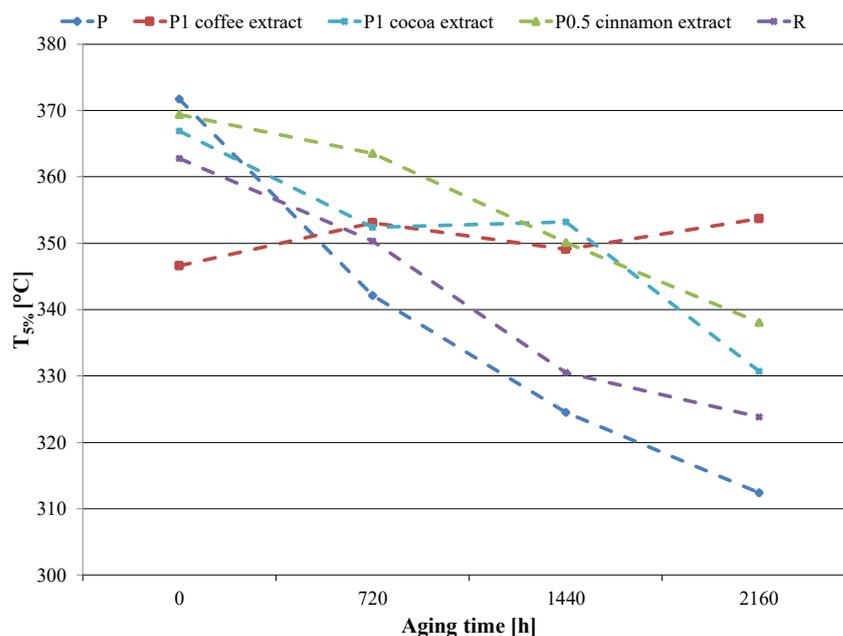
**Figure 6.** The temperature of 5% weight loss ( $T_{5\%}$ ) values of selected samples as a function of aging time.
