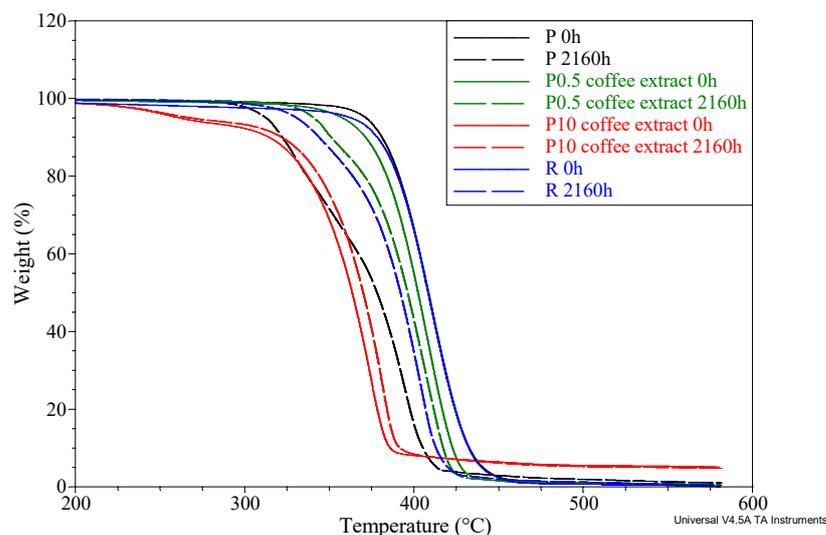
Figure 5. TG curves of selected samples before and after the aging process.
