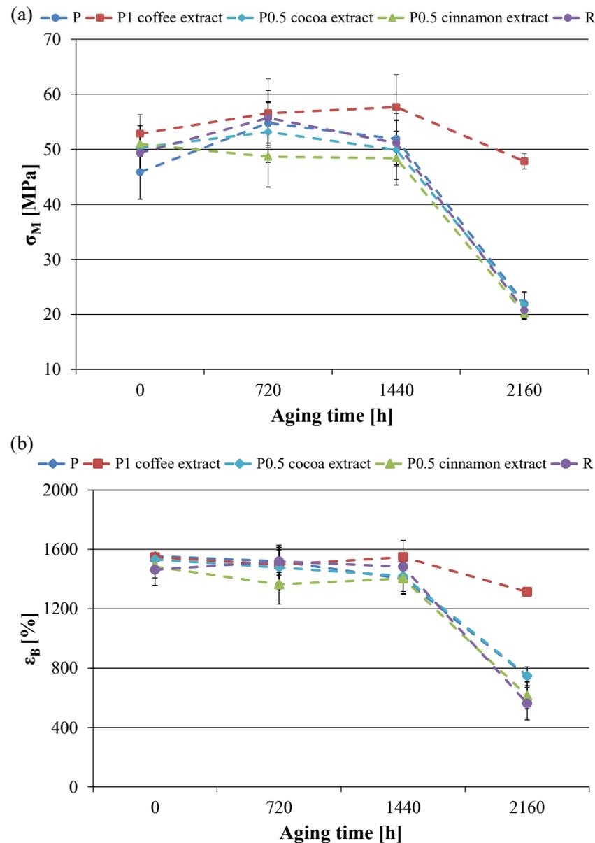
**Figure 4.** Values of (a) tensile strength ( $\sigma_M$ ) and (b) strain at break ( $\epsilon_B$ ) of selected samples as a function of aging time.
