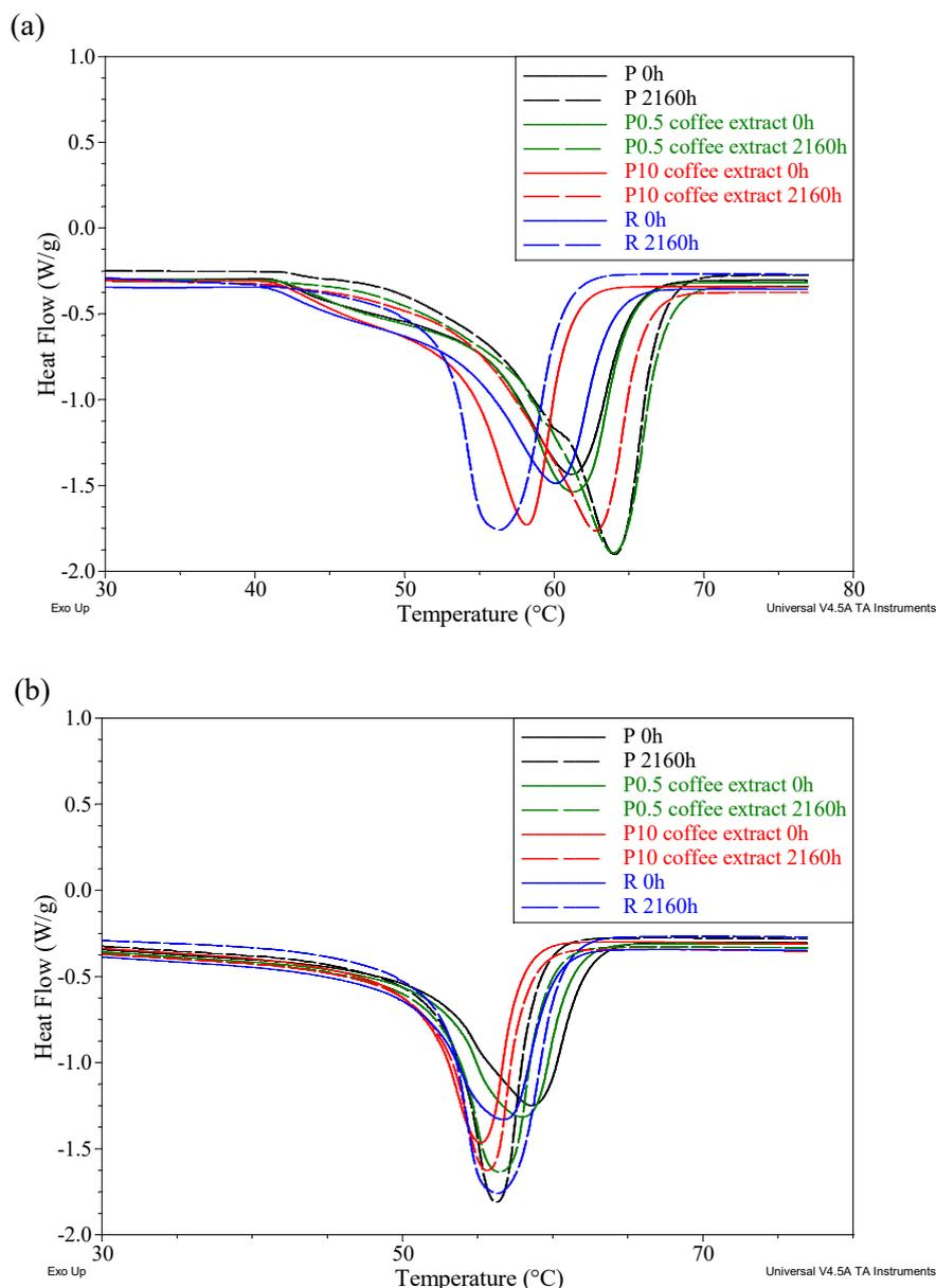
**Figure 7.** DSC curves of unaged and aged samples containing coffee extract; (a) first heat (b) second heat.
