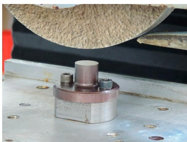
**Figure 4.** View of a ground C45 steel specimen mounted on an oscillating table.
