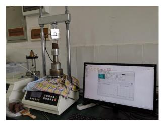
Figure 1. The TSZ series fully automatic triaxial instrument.
