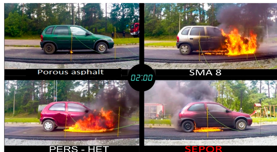
Figure 35. Fire development 120 s after ignition.
