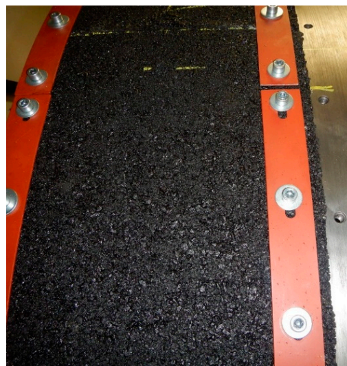
Figure 31. SEPOR plates mounted on the drum.
