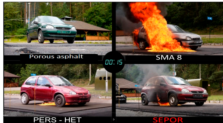
Figure 34. Fire development 15 s after ignition.
