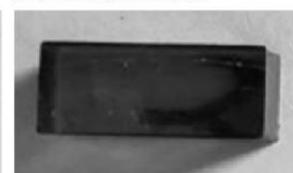
**Figure 10.** Test samples of cured unsaturated polyester resin.
