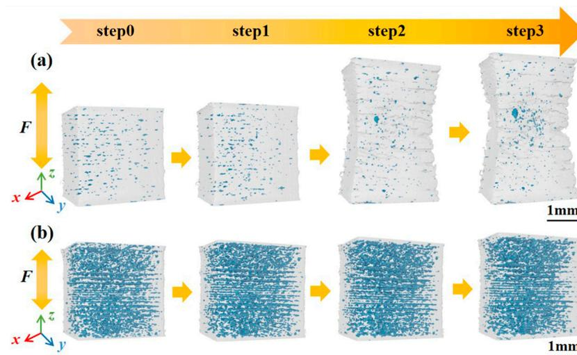
**Figure 3.** Volume renderings of VOI2 at different loading steps: (a) Specimen 400 and (b) Specimen 1000.
