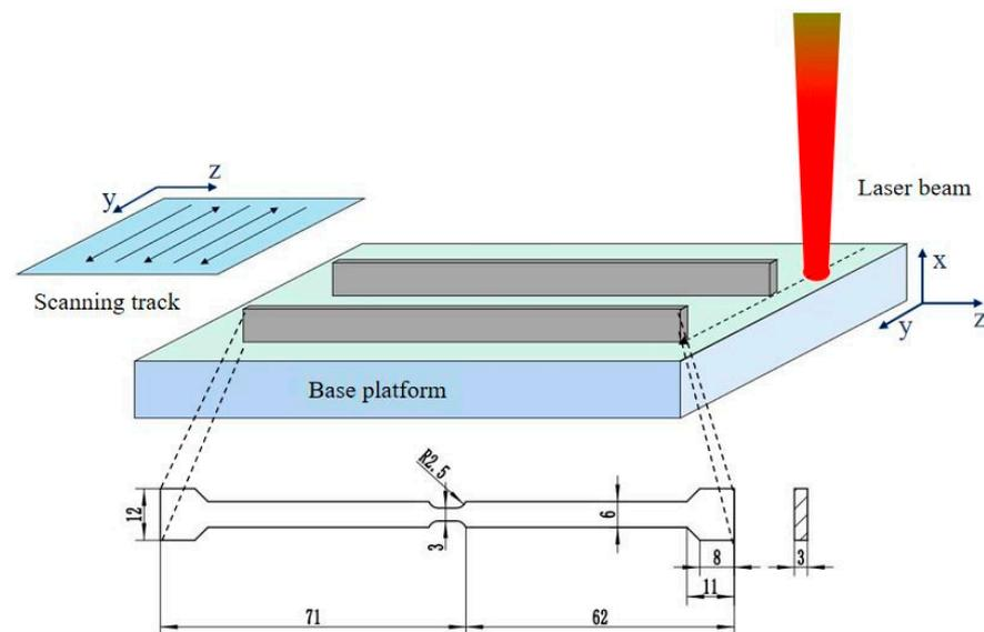
**Figure 1.** The detailed preparation process and dimensions of Invar 36 alloy specimens.
