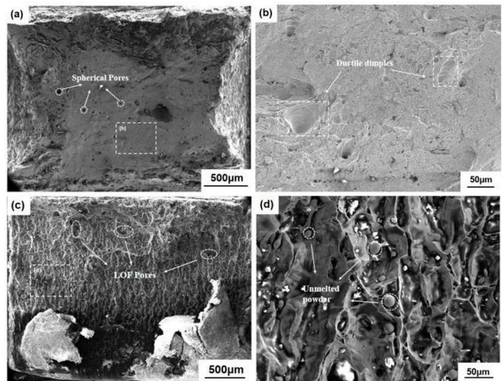
**Figure 11.** Fracture morphology of (a,b) Specimen 400 and (c,d) Specimen 1000 obtained by SEM.
