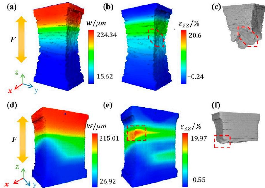
**Figure 10.** The displacement ( $W$ ) field, uniaxial strain ( $\epsilon_{zz}$ ) field and 3D rendering image of fracture of the VOI1 in (a–c) Specimen 400 and (d–f) Specimen 1000.
