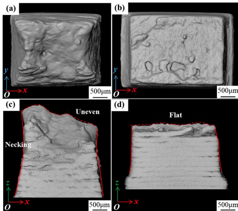
Figure 6. Fracture morphology of (a,c) Specimen 400 and (b,d) Specimen 1000 obtained by XCT reconstruction.
