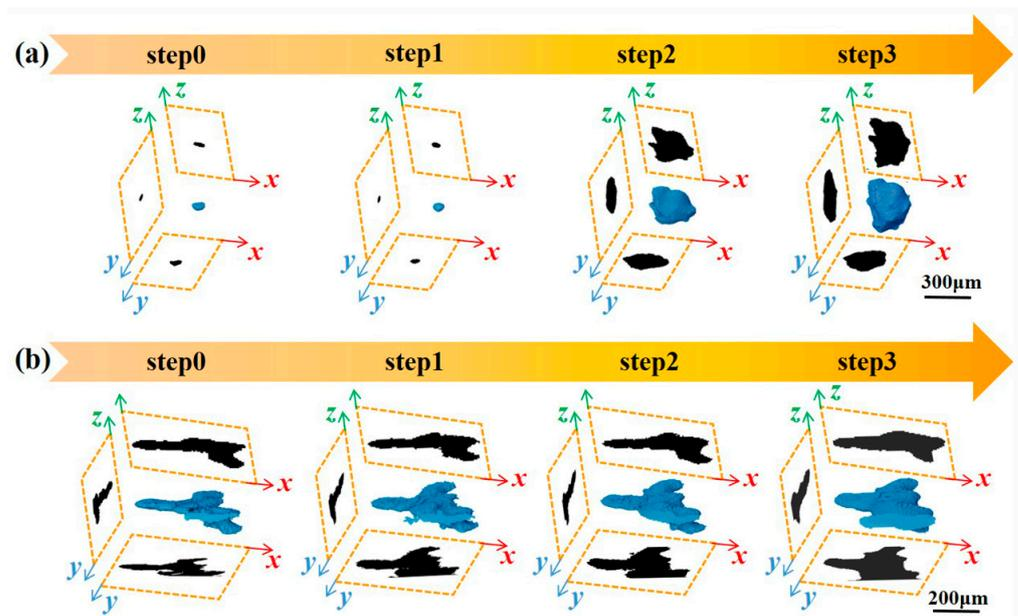
**Figure 9.** Three dimensional morphology of the critical defects of (a) Specimen 400 and (b) Specimen 1000 at different loading steps.
