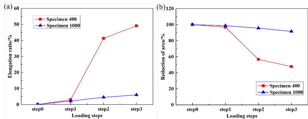
**Figure 7.** (a) Elongation ratios at different loading steps; (b) reductions of the area at different loading steps.
