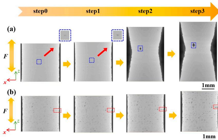
Figure 5. Visualization of critical defect evolution in gauge sections for (a) Specimen 400 and (b) Specimen 1000.
