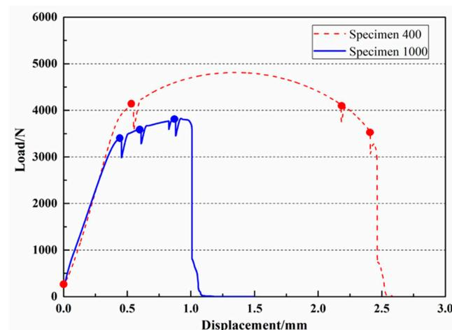
**Figure 2.** Load-displacement curves for the specimens fabricated at different scanning speeds.
