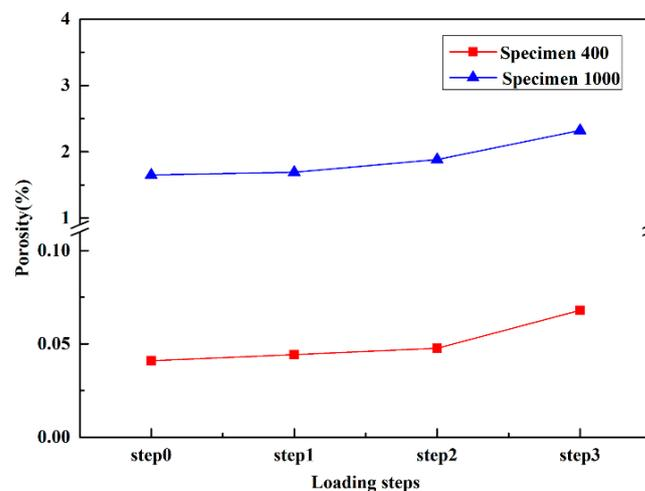
**Figure 4.** Porosity evolution of Specimen 400 and Specimen 1000 at different loading steps.
