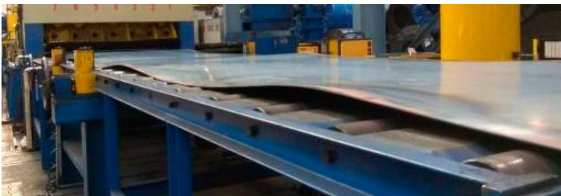
**Figure 2.** The sheet metal edge and longitudinal waviness examples after unwinding from the coil of S235JR + AR steel grade with dimensions of 3 × 1500 mm.
