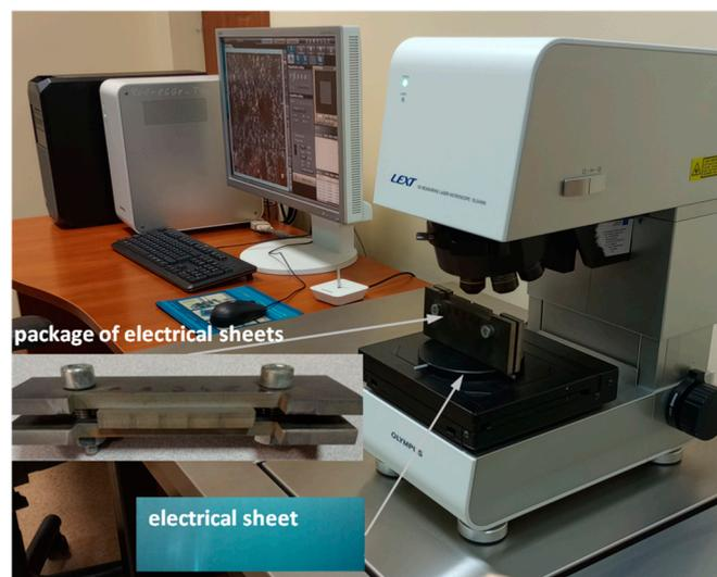
**Figure 2.** Station for measuring the geometric structure of the surface—LEXT OLS4000 laser confocal microscope from OLYMPUS.
