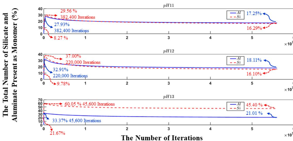
**Figure 6.** The change in the number of aluminate and silicate monomers present in the system during 56 million iterations for the different pHs. Metakaolinite particles are considered monomers only when dissolved according to the dissolution process.
