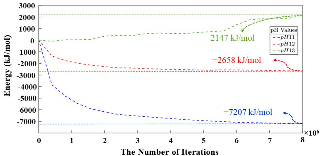
**Figure 4.** Energetic evolution of silicate particles in solution obtained for pH systems of 11, 12, and 13, where metakaolinite is not yet involved.
