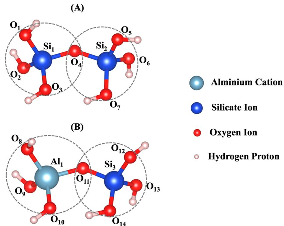
**Figure 2.** Dimerization reaction based on tetrahedron formation for (A) Si-O-Si and (B) Si-O-Al optimized by the DFT computational approach. Tables A1 and A2 in Appendix A show bond lengths and angles between atoms. The radius of coarse-grained particles equals the averaged bond length. The two particles touch at a single point, either the center of bonding oxygen, O4 (case (A)) or O11 (case (B)).
