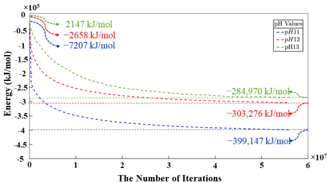
**Figure 5.** The equilibrium condition for three different pH systems was obtained through energy minimization computation of the silicate particles (starting at 0 iterations) and metakaolinite for 8 million iterations. The point at which metakaolinite is introduced to the system is denoted at iteration 0. Thus, pre-equilibration takes place for additional “8,000,000” iterations (shown in Figure 3).
