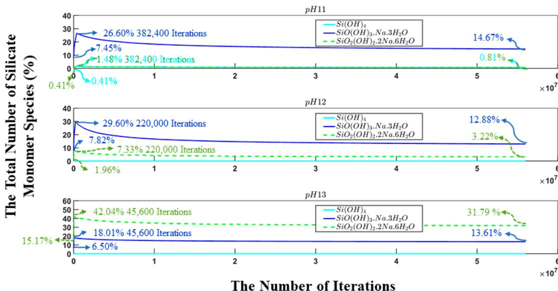
**Figure 7.** The evolution of the number of silicate monomers present in the system during 56 million iterations. At the start of the simulation (at iteration zero), metakaolinite particles were not included as they were undergoing the dissolution process.
