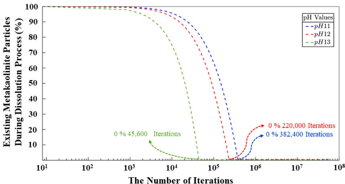
Figure 10. Dissolving process of metakaolinite during 56 million iterations.
