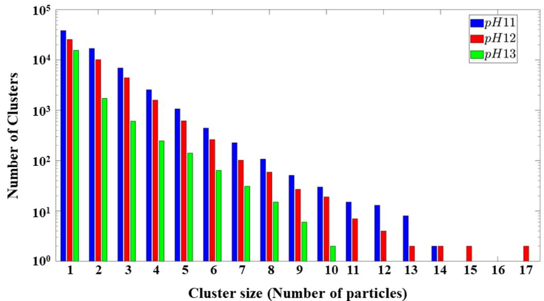
**Figure 14.** Cluster distribution. The y-axis shows the total number of clusters, and the x-axis describes the number of particles in each cluster. The clusters that have a particle count of 1 are the monomers in the system.
