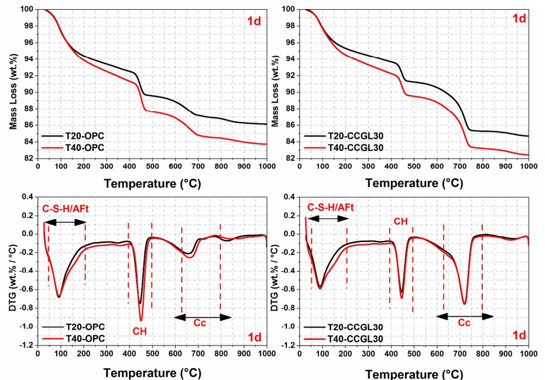
Figure 7. TG-DTG curves of hardened pastes at 1 day.
