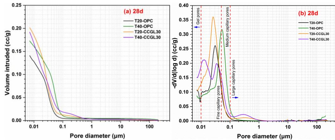
Figure 12. (a) Cumulative and (b) incremental pore volume of hardened pastes at 28 days.
