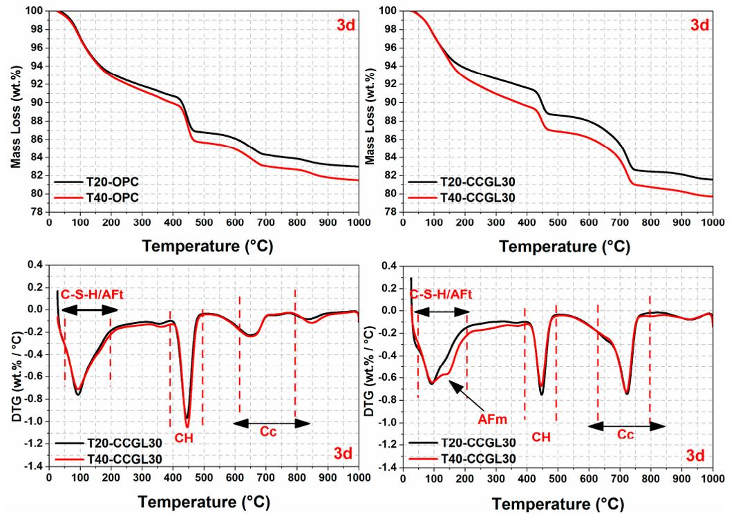
Figure 8. TG-DTG curves of hardened pastes at 3 days.
