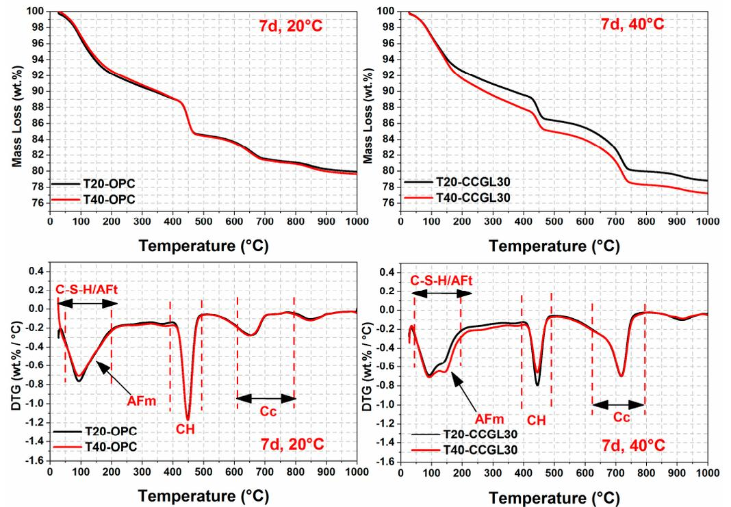
Figure 9. TG-DTG curves of hardened pastes at 7 days.
