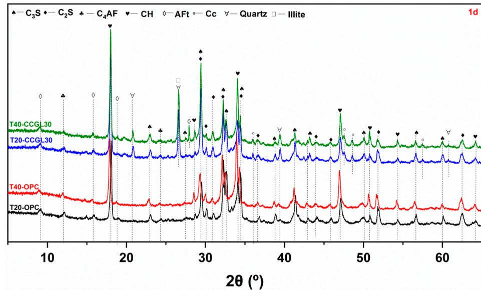
**Figure 3.** XRD patterns of paste samples cured at 20 and 40 °C at 1 d ( $C_3S$ : tricalcium silicate,  $C_2S$ : dicalcium silicate,  $C_4AF$ : ferrite, CH: portlandite, AFt: ettringite, Cc: calcite).
