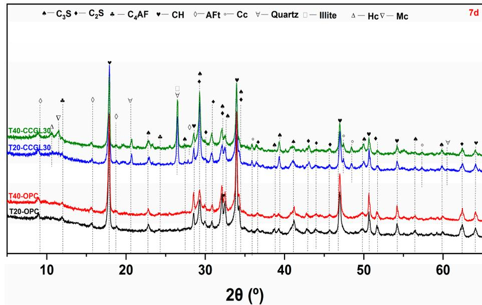
**Figure 5.** XRD patterns of paste samples cured at 20 and 40 °C at 7 d ( $C_3S$ : tricalcium silicate,  $C_2S$ : dicalcium silicate,  $C_4AF$ : ferrite, CH: portlandite, AFt: ettringite, Cc: calcite).
