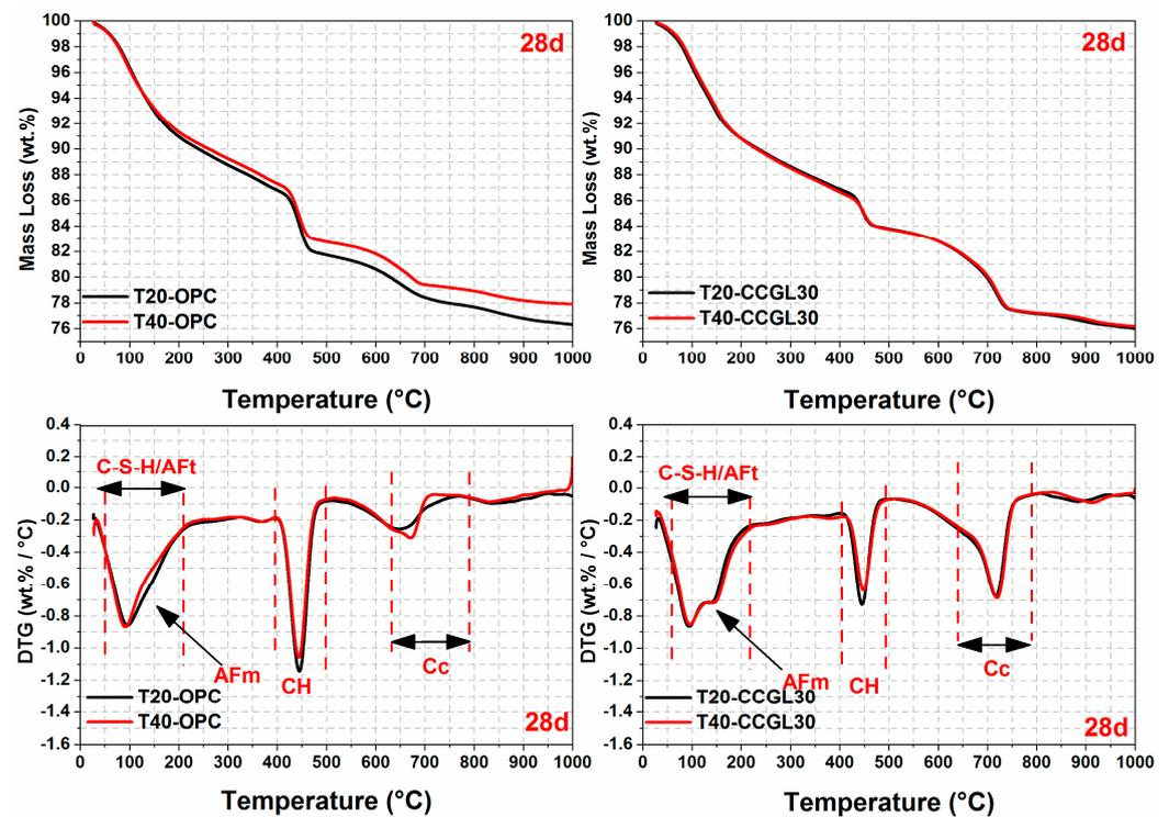
Figure 10. TG-DTG curves of hardened pastes at 28 days.
