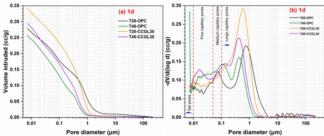
Figure 11. (a) Cumulative and (b) incremental pore volume of hardened pastes at 1 d.
