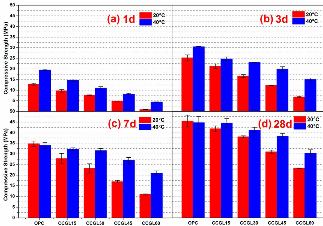
**Figure 2.** Compressive strength of mortar samples cured at 20 and 40 °C up to 28 d.
