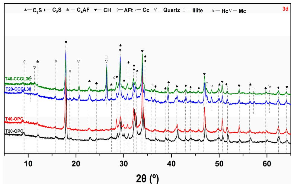
**Figure 4.** XRD patterns of paste samples cured at 20 and 40 °C at 3 d ( $C_3S$ : tricalcium silicate,  $C_2S$ : dicalcium silicate,  $C_4AF$ : ferrite, CH: portlandite, AFt: ettringite, Cc: calcite).
