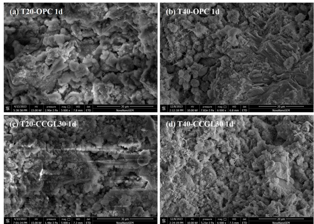
Figure 13. SEM observation of hardened pastes at 1 d.
