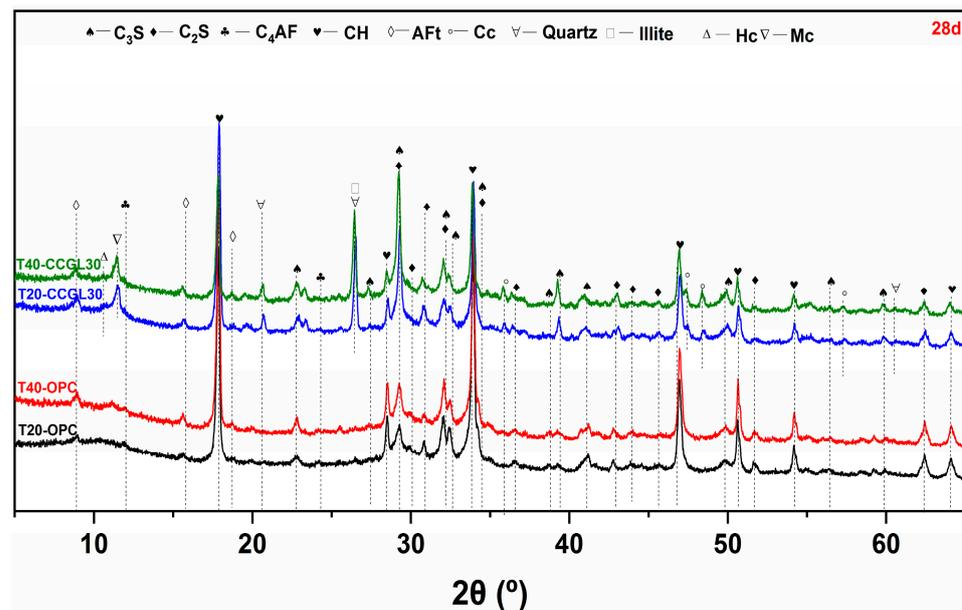
**Figure 6.** XRD patterns of paste samples cured at 20 and 40 °C at 28 d ( $C_3S$ : tricalcium silicate,  $C_2S$ : dicalcium silicate,  $C_4AF$ : ferrite, CH: portlandite, AFt: ettringite, Cc: calcite).
