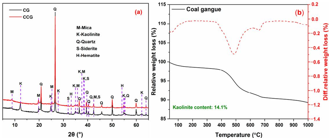
**Figure 1.** (a) XRD patterns and (b) TG/DTG curves of CG and CCG.
