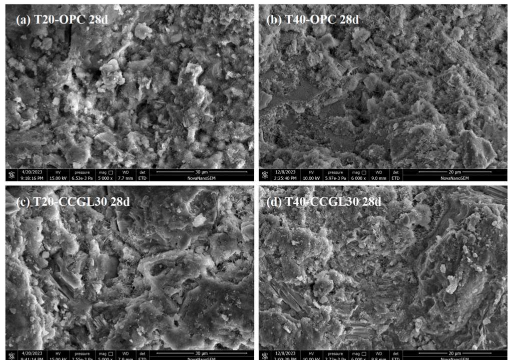
Figure 14. SEM observation of hardened pastes at 28 d.
