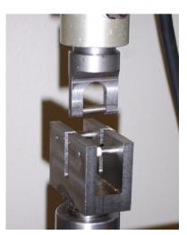
Figure 5. 3-point flexural beam test fixture in loadframe. Test span is 45.4 mm.
