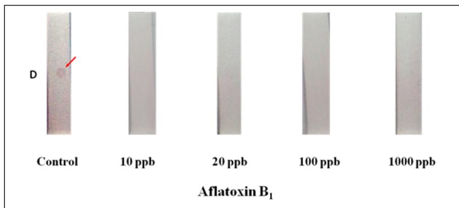
**Figure 5.** Cross reactivity of AFB1 test strip. The Ochratoxin A (OTA) test solution was analyzed by AFB1 test strip. Details of the preparation of the lateral flow test device and assay are described in the text. Binding inhibition is shown in the presence of AFB1.
