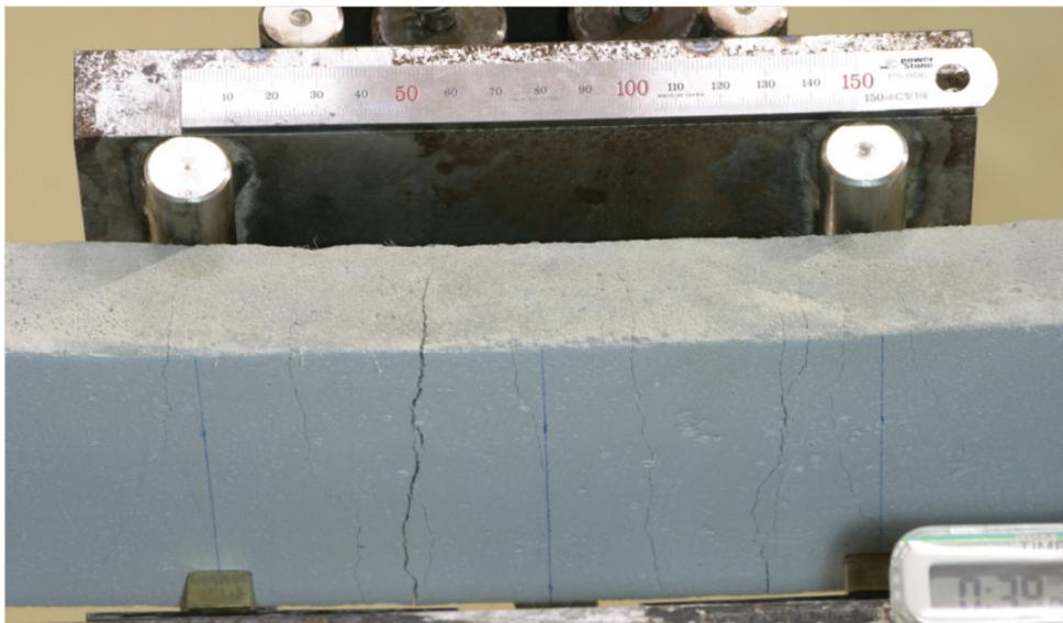
Static test results indicate that the mixture used in this study shows the unique behaviors of ductile HPFRCC or ECC. The specimens sustained the load continuously, even after peak load, and strain hardening behavior was observed with finely distributed microcracks in flexural tests.
