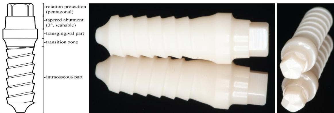
**Figure 1.** The evaluated implant system (zit-z, Ziterion GmbH, Uffenheim, Germany) and its metrics used for the experiment: 4.0 mm diameter, 13 mm intraosseous length, 2.5 mm transgingival height, 4 mm abutment height (pentagonal and tapered part).
