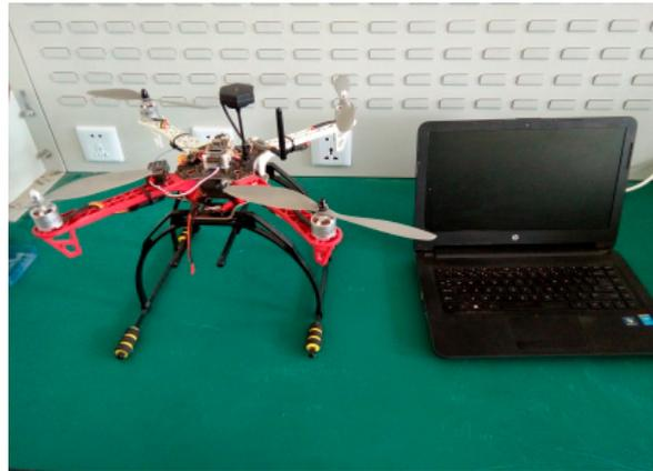
Figure 5. The quadrotor used in the experiments.
