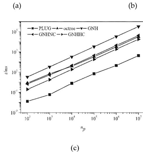
**Figure 12.** Scalability of the different methods with regard to the increasing number of the particles on the different types of meshes. (a) Hexahedral mesh; (b) Tetrahedral mesh; (c) Polyhedral mesh.
