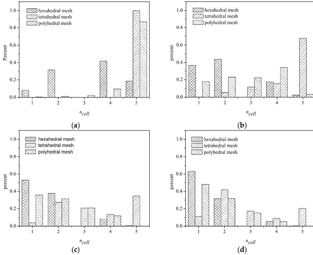
**Figure 11.** The percentage of background cubes covered by a given number of computational cells. (a) Background grid with  $100^3$  cells; (b) Background grid with  $200^3$  cells; (c) Background grid with  $300^3$  cells; (d) Background grid with  $400^3$  cells.
