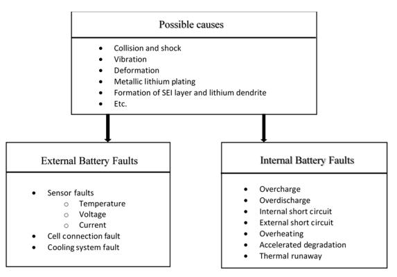
Figure 1. Internal and external Lithium-ion (Li-ion) battery faults and their causes.
