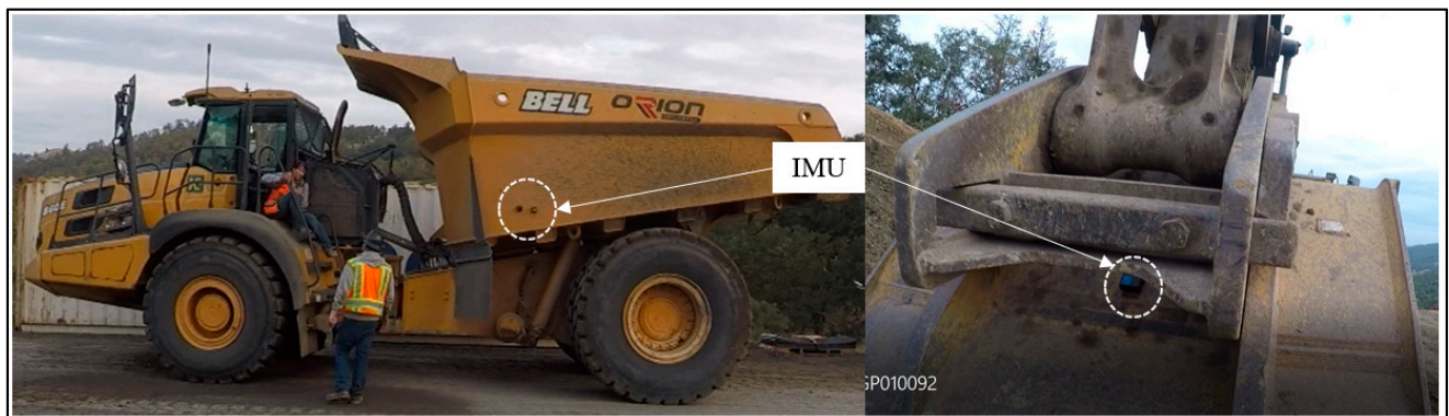
Figure 6. IMU attachment to dump truck and excavator.
