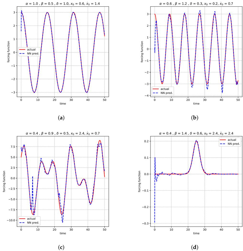
**Figure 4.** Figure shows the agreement between neural network predictions and actual forcing functions: (a) sinusoidal (b) sinusoidal with increased non-linearity and frequency (c) sum of two sinusoidal (d) impulse for duffing’s equation.
