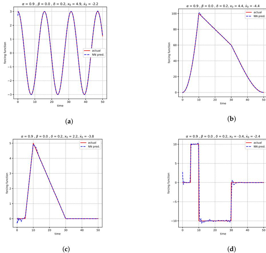
**Figure 5.** Figure shows the agreement between neural network predictions and actual forcing functions: (a) sinusoidal (b) combination of parabolic, linear and cubic (c) triangular (d) step for spring mass damper system.
