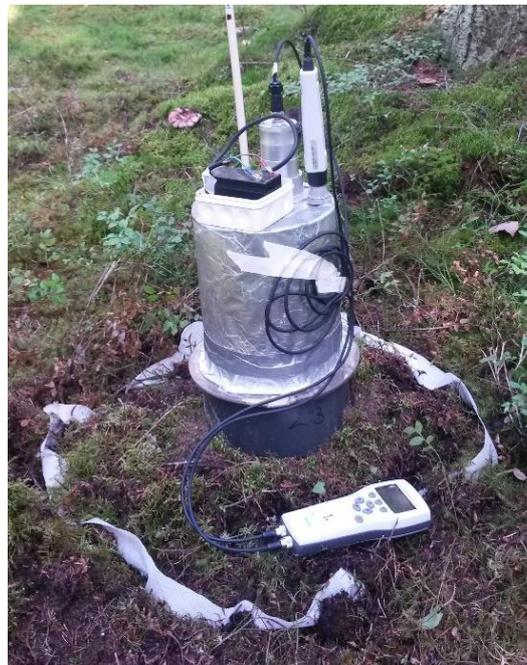
**Figure 2.** Soil surface respiration chamber darkened with aluminum foil and containing the CARBOCAP® GMP343 CO<sub>2</sub> probe and a data logger on the ground in front. The measurement point is one of the trenched measurement points. Photo: Maiju Kosunen.
