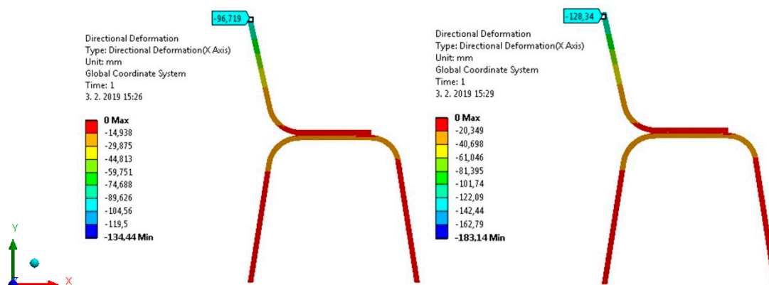
Figure 7. FEM visual outputs of deformation and displacement of the back while the load is applied. Left figure for 110 kg and right figure for 150 kg.
