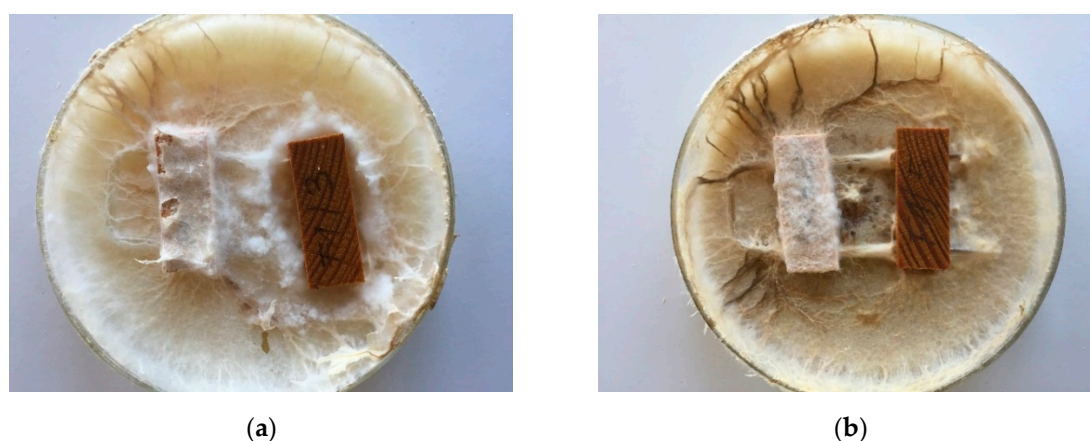
Figure 1. Scots pine wood after exposure to C. puteana : (a) control wood sample and wood treated with 18.9% propolis extract; (b) control wood sample and wood treated with 30% propolis extract.
