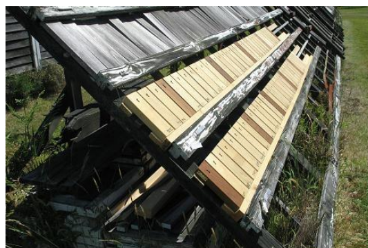
Figure 4. Flat panel test after installation. The upper rail holding the screws is H3-treated radiata pine. The lower L-shaped rail is untreated radiata pine.
