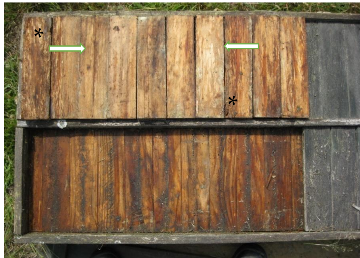
Figure 6. Double layer test after 10 years exposure. The upturned samples 3rd–7th from left, upper row) are copper-chrome arsenate (CCA)-treated (between two arrows), all others are untreated controls. The upper surface of the second layer opposite in the lower row is the same treatment. Note that there is very little decay in the CCA treated samples but there is severe decay in all of the untreated samples (examples of visible decay are indicated by asterisk * symbol).
