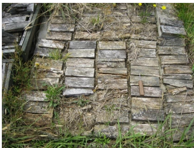
Figure 5. Ground proximity test after 10 years exposure. The samples were originally covered with shade cloth but this was damaged and debris from mowing the surrounding grass supported vegetation growth between and on samples. Most of the samples, including preservative-treated, ones were in poor condition.
