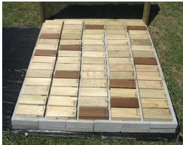
Figure 1. Ground proximity test at installation with the shade-cloth and frame removed. The samples are placed on two layers of 40 mm thick pumice slabs with plastic weed mat underneath.
