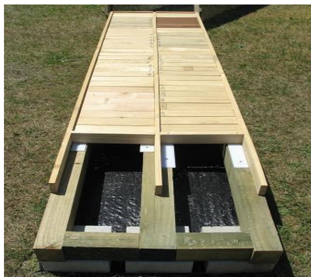
Figure 2. Double layer test at installation. 100 mm square bearers supported on concrete blocks with plastic weed cloth underneath. The plastic strips between the samples and bearers were removed after a few weeks exposure. The batten along the centre was untreated pine, those on the outside were H3 treated. The whole assembly was surrounded by a 300-mm-deep frame covered with shade cloth.
