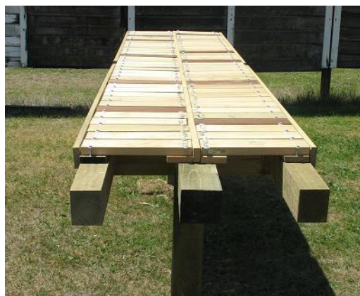
Figure 3. Raised decking test at installation showing treated bearers and battens at the outer ends of the samples and untreated bearers plus separating strip in the centre. For the ground-level decking test, the treated bearers were placed directly on the ground, but other details were the same as for raised decking.
