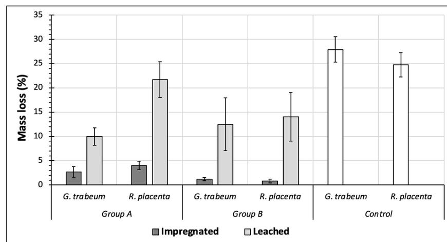
Figure 6. Mass loss, expressed in percent, in impregnated and leached specimens of radiata pine wood treated with CuNP after exposure to *Gloeophyllum trabeum* and *Rhodonia placenta*. The maximum standard error for mass loss is 3.6%.
