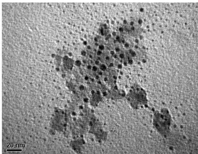
**Figure 1.** Transmission electron microscope image of copper nanoparticles used in this study.
