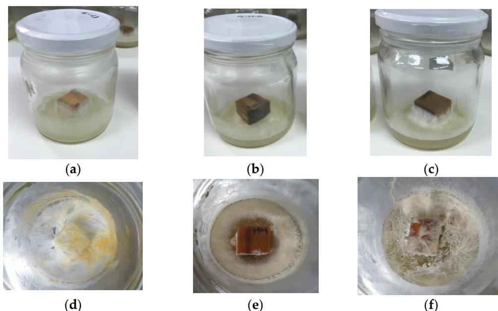
**Figure 7.** Photographs of radiata pine samples exposed to biodeterioration. (a,d) control sample; (b,e) sample impregnated with CuNPs; and (c,f) leached sample. Images (a–c) correspond to samples at week 4 of exposure to *G. trabeum*. Images (d–f) correspond to samples at week 16 of exposure to *G. trabeum*.
