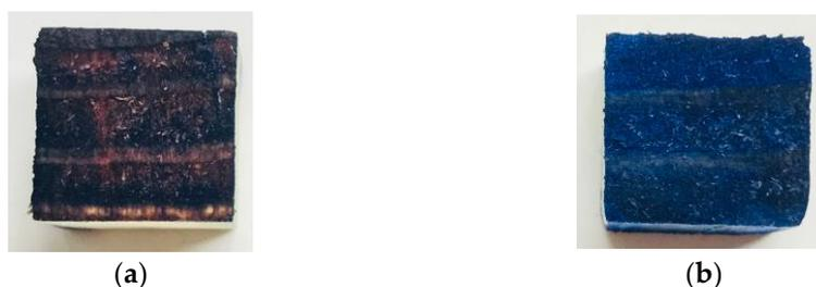
**Figure 2.** Photographs of interior cross-section of impregnated wood samples with CuNPs with chromium azurol staining. (a) Group A sample impregnated with 1 g/L CuNPs and (b) group B sample impregnated with 3 g/L CuNPs.
