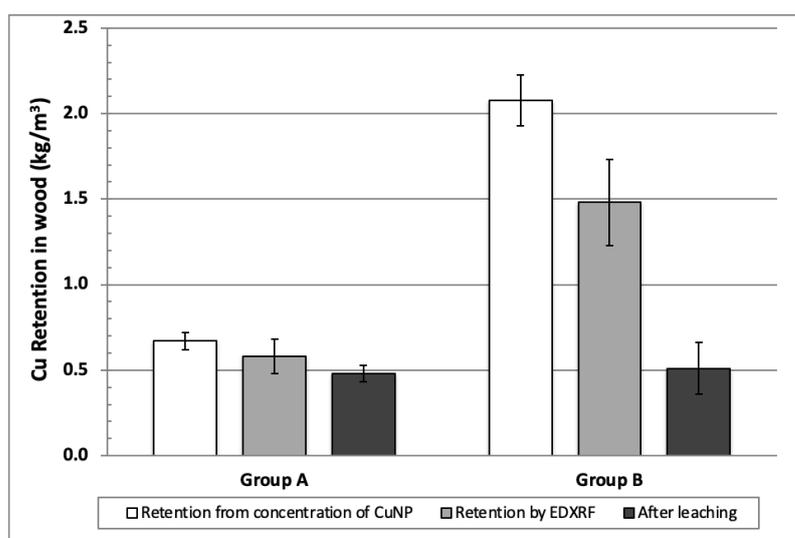
**Figure 3.** Copper retention in radiata pine wood impregnated with CuNPs. Group A woods were treated with a 1 g/L solution of CuNP and group B woods were treated with a 3 g/L solution of CuNP. White bars correspond to Cu retention in wood from the concentration of CuNPs in the solution, gray bars correspond to Cu retention in wood impregnated by EDXRF, and black bars correspond to Cu retention in wood leached by EDXRF.
