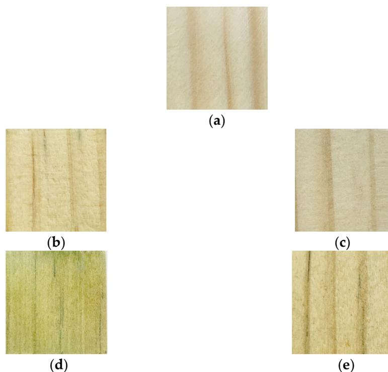
**Figure 4.** Photographs of control, impregnated, and leached radiata pine wood samples. (a) Control sample; (b) group A, wood impregnated with CuNP 1 g/L and (c) leached; (d) group B, wood impregnated with CuNP 3 g/L and (e) leached.
