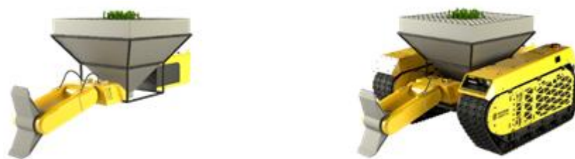
Figure 3. Planting payload (left) and planting payload with the UGV (right).
