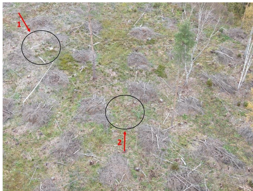
Figure 6. Detection of different objects (1—stumps, roots, deadwood, slash) and suitable planting spots (2) in clear-cut area using UAV imagery.
