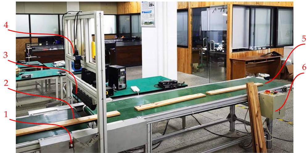
**Figure 1.** Image acquisition device: (1) photoelectric sensor, (2) solid wood board, (3) linear light source, (4) CCD camera, (5) belt conveyor, and (6) sample solid wood floorboard.
