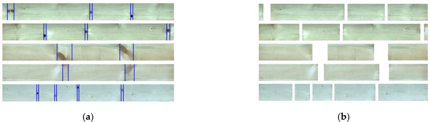
**Figure 5.** Defect removal. (a) The cutting points of defects. (b) Segments after removing defects.
