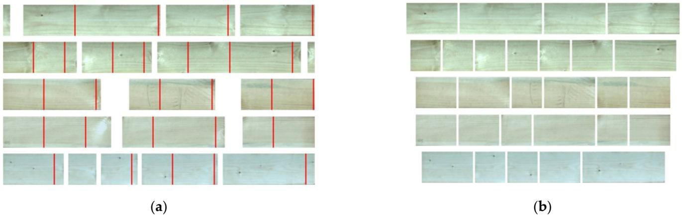
**Figure 6.** Elite retention genetic algorithm sawing results. (a) Planned cutting points. (b) Wood after sawing.
