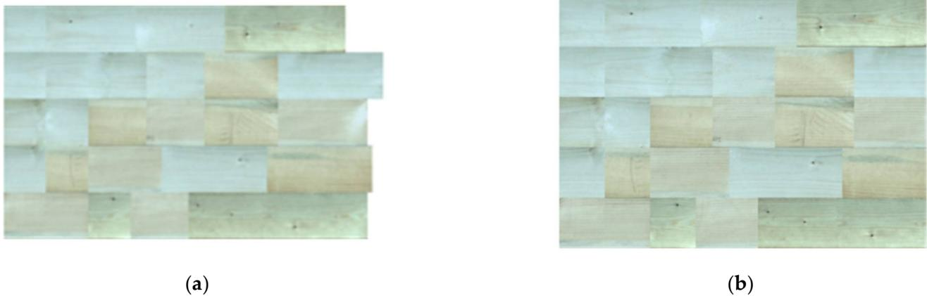
**Figure 7.** The layout of wood splicing board with standardized pieces. (a) Board spliced by row. (b) Rectangular board.
