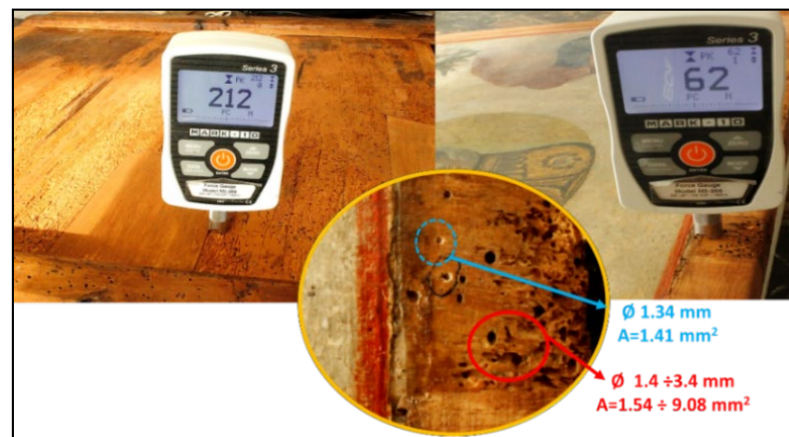
Figure 12. Comparison of the trace of the measuring tip with the flight hole caused by xylophagous insects: Mark 10 tip, Ø 1.34 mm A = 1.41 mm 2 , flight hole, Ø 1.4–3.4 mm, A = 1.54–9.08 mm 2 .
