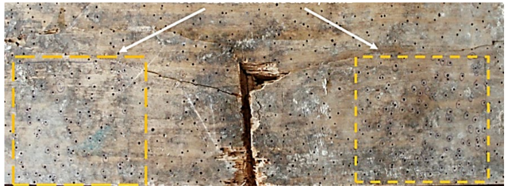
Figure 6. Marking and counting of flight holes per dm 2 .
