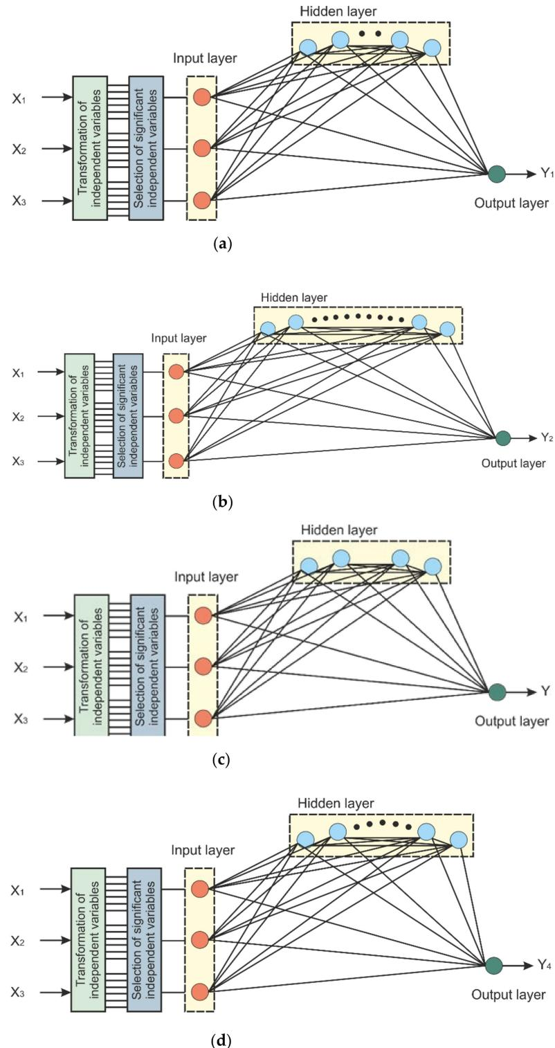
**Figure 1.** The optimum structure of developed cascade ANN models that could predict the: (a) delamination factor at the outlet; (b) delamination factor at the inlet; (c) thrust force; (d) drilling torque.
