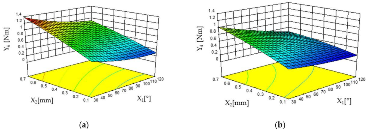
**Figure 6.** The 3D plots showing interaction effects of the drill tip angle ( $X_1$ ) and tooth bite ( $X_2$ ) on the drilling torque ( $Y_4$ ) when the holes were 'performed' with a flat drill (a) and with a helical drill (b).
