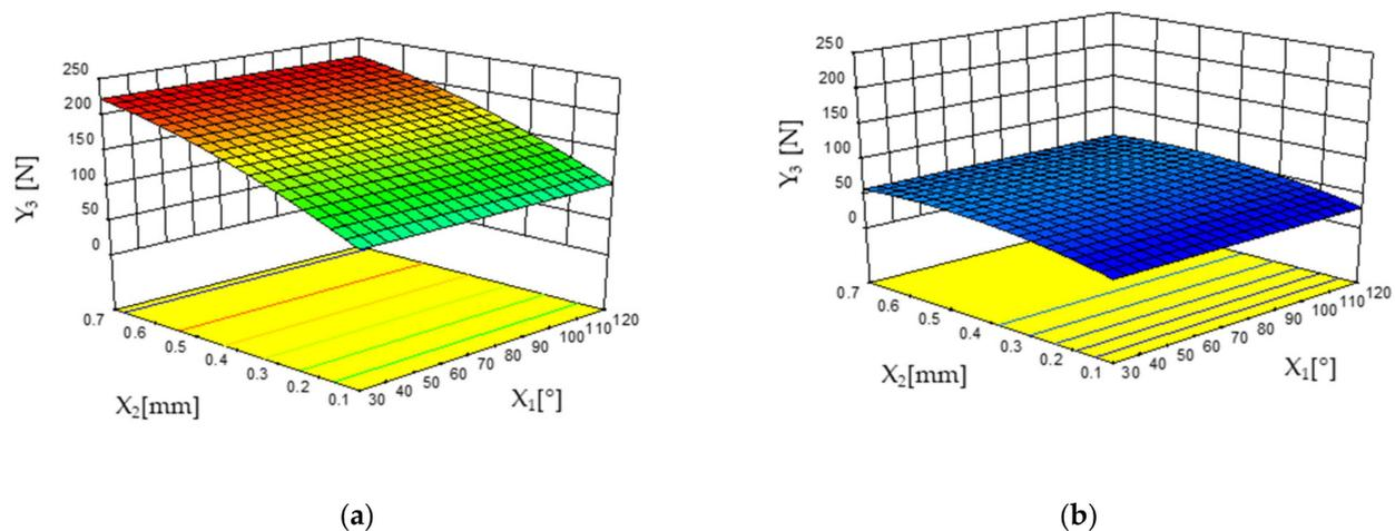
**Figure 5.** The 3D plots showing interaction effects of the drill tip angle ( $X_1$ ) and tooth bite ( $X_2$ ) on the thrust force ( $Y_3$ ) when the holes were ‘performed’ with a flat drill (a) and with a helical drill (b).
