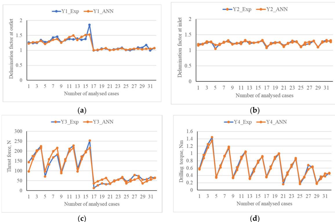
**Figure 2.** Comparison between predicted vs. experimental values: (a) delamination factor at the outlet; (b) delamination factor at the inlet; (c) thrust force; (d) drilling torque.
