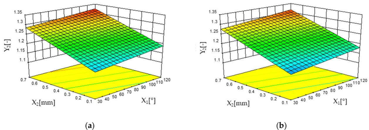
**Figure 4.** The 3D plots showing interaction effects of the drill tip angle ( $X_1$ ) and tooth bite ( $X_2$ ) on the delamination factor at the inlet ( $Y_2$ ) when the holes were ‘performed’ with a flat drill (a) and with a helical drill (b).
