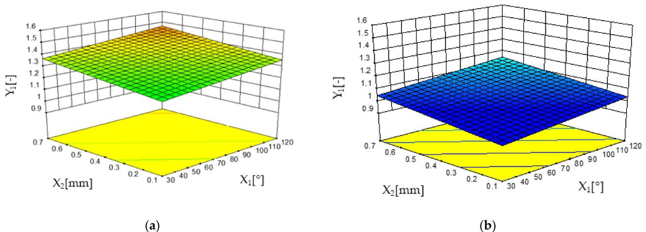
**Figure 3.** The 3D plots showing interaction effects of the drill tip angle ( $X_1$ ) and tooth bite ( $X_2$ ) on the delamination factor at the outlet ( $Y_1$ ) when the holes were ‘performed’ with a flat drill (a) and with a helical drill (b).
