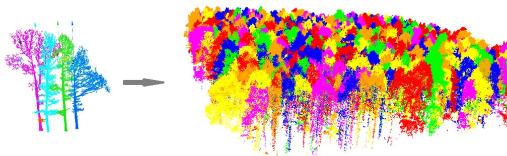
**Figure 6.** The results of segmentation algorithm: the left shows the algorithm demonstration of a small batch of samples, and the right figure shows part of the segmentation results, which is rendered into different colors to distinguish individual trees.
