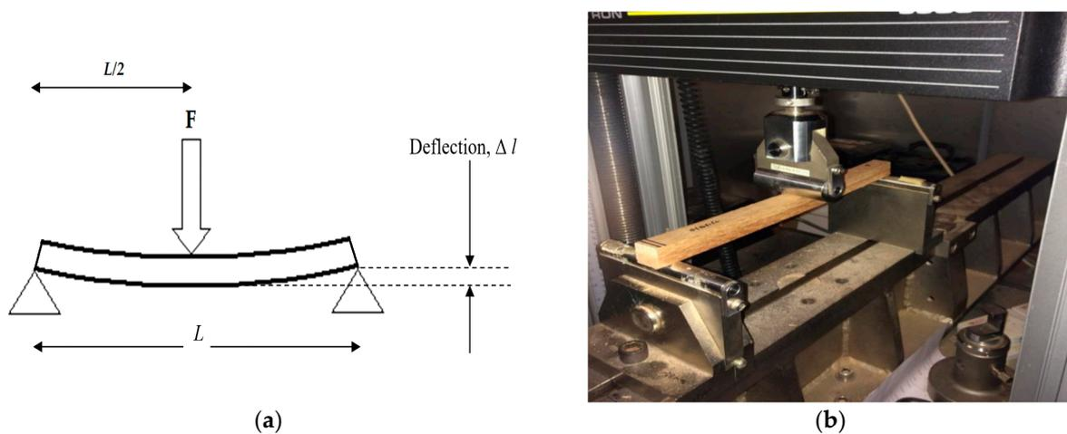
Figure 3. (a) The static bending test [24]; (b) the static bending test at the laboratory.
