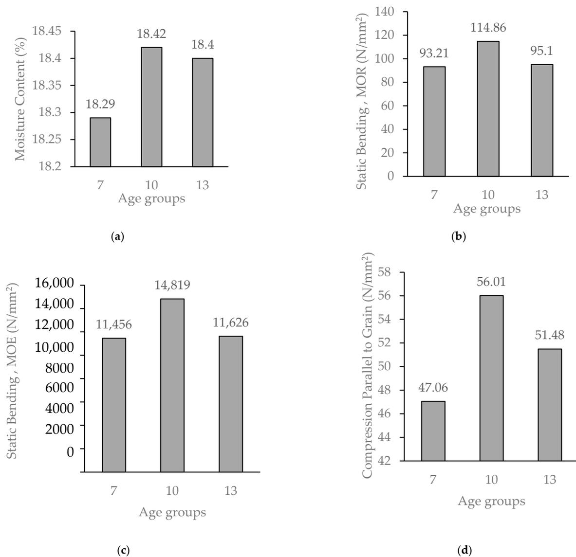
**Figure 9.** (a) Moisture content; (b) static bending, MOR; (c) static bending, MOE; (d) compression parallel to grain results of untreated *Acacia mangium* superbulk [22].
