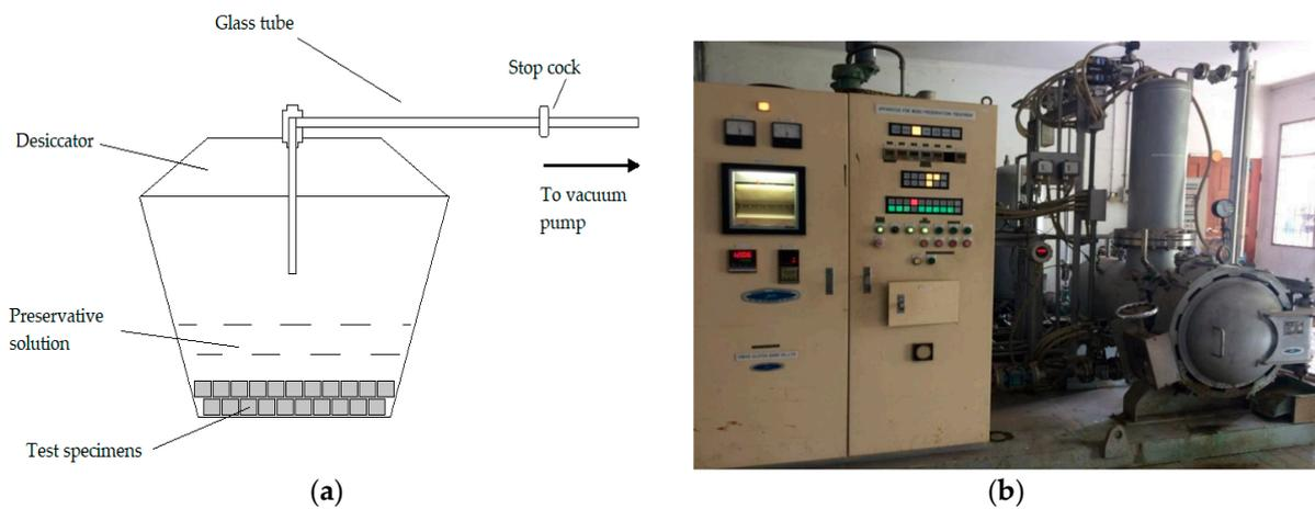
**Figure 6.** (a) The treatability test vacuum desiccators setup [13]; (b) treatment process machine.
