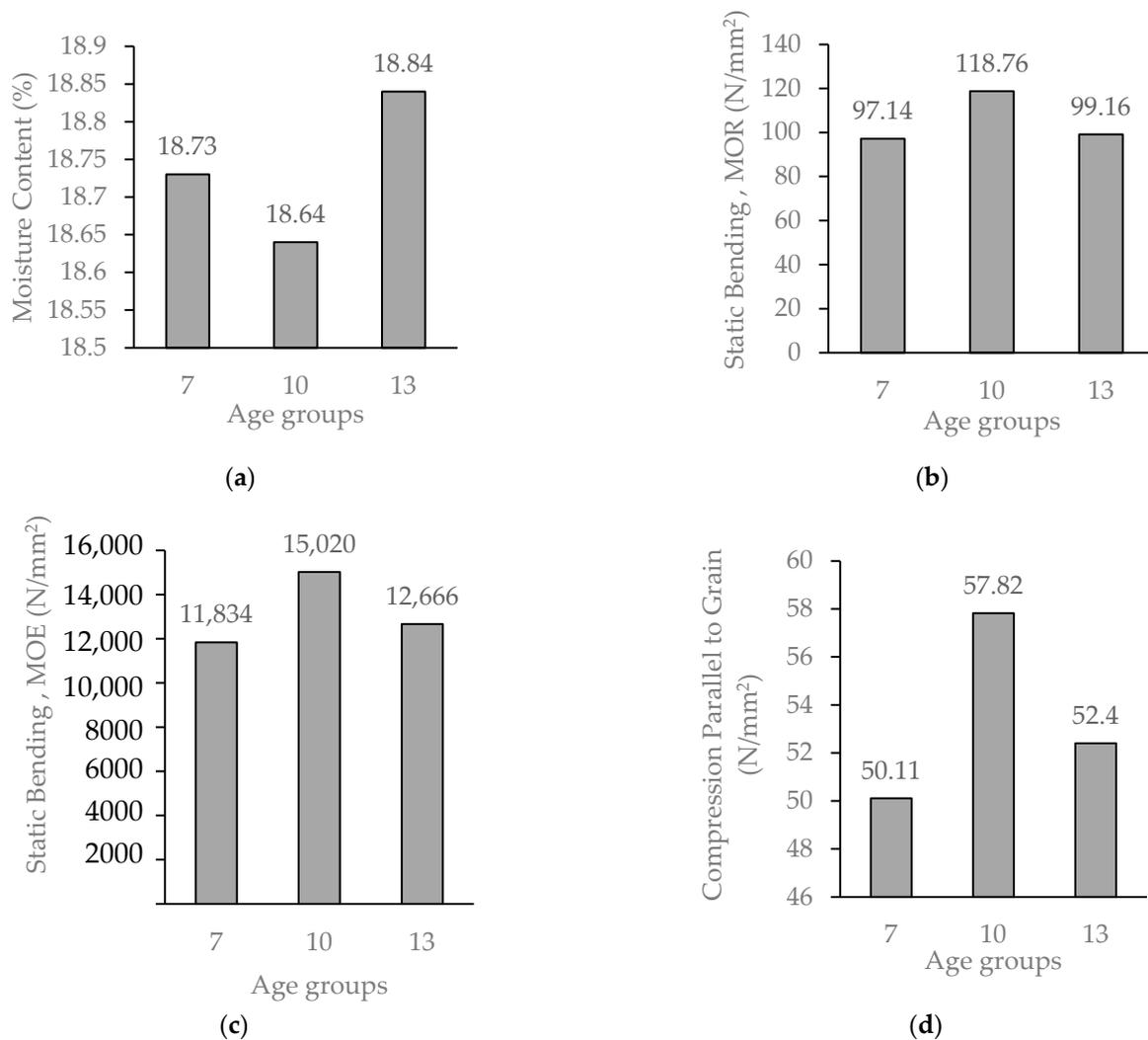
**Figure 8.** (a) Moisture content; (b) static bending, MOR; (c) static bending, MOE; (d) compression parallel to grain results of treated *Acacia mangium* superbulk.
