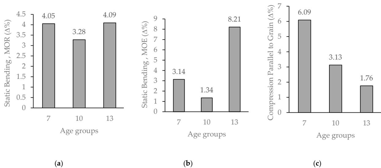
**Figure 10.** (a) Static bending, MOR; (b) static bending, MOE; (c) compression parallel to grain results of percentage increment between treated and untreated *Acacia mangium* superbulk.
