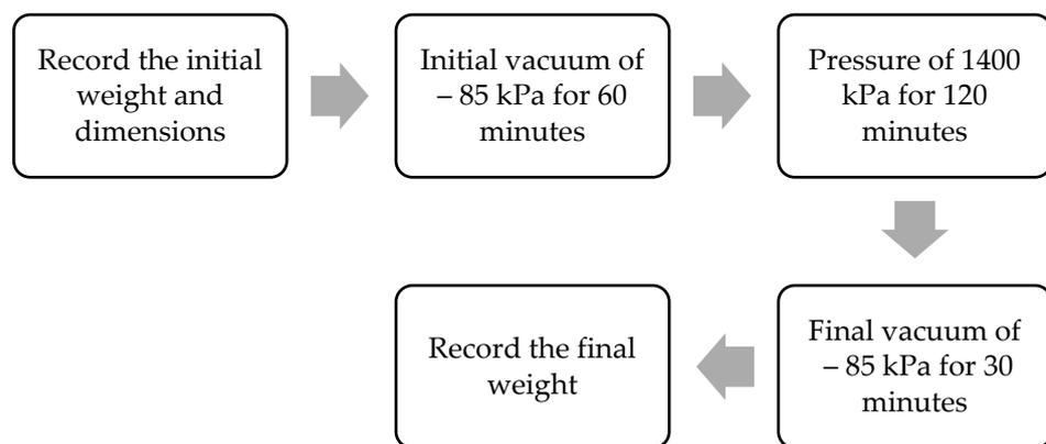
**Figure 7.** The flowchart for the treatment process.
