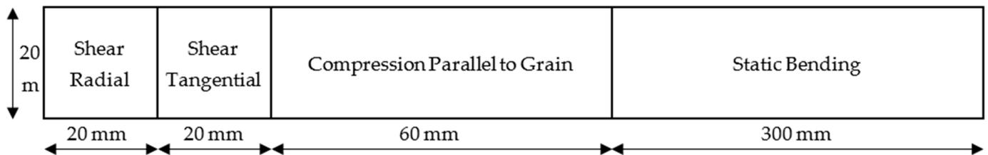
Figure 2. The dimensions for mechanical strength testing.
