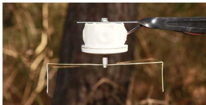
**Figure 1.** Running spore trap (ROTTRAP 120) coated with double-sided tape on the impaction side of the square section wire.
