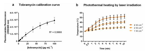
**Figure S3.** (a) Tobramycin calibration curve by measuring the fluorescamine fluorescence of a series of tobramycin concentrations (1–100  $\mu$ g mL<sup>-1</sup>) by a fluorescence plate reader (355/460 nm) and fitting into a quadratic curve (mean  $\pm$  SD) (b) Photothermal heating curve of GQD-tobramycin particles using a 980 nm continuous wave laser at 1, 2 and 4 W cm<sup>-2</sup> (mean  $\pm$  SD).
