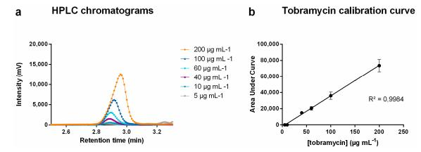
**Figure S1.** Tobramycin calibration curve by measuring the tobramycin content by HPLC-UV. (a) A series of tobramycin solutions ranging from 5–200  $\mu$ g mL<sup>-1</sup> was analyzed by HPLC-UV. (b) The standard curve was generated by plotting the Area Under Curve (AUC) to the corresponding tobramycin concentration and fitting to a linear curve (average  $\pm$  SD).
