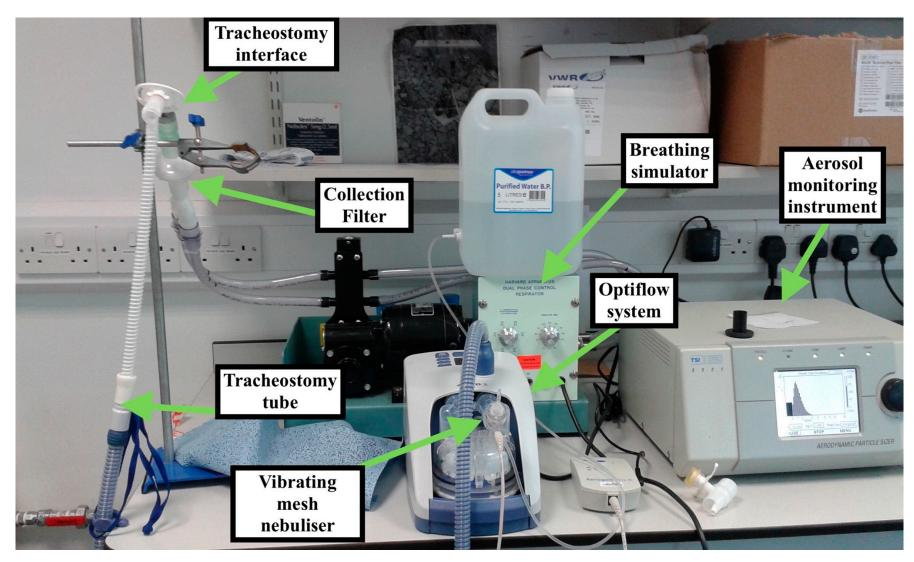
Figure S3. A photograph highlighting the physical setup for the adult and paediatric tracheotomy set up.
