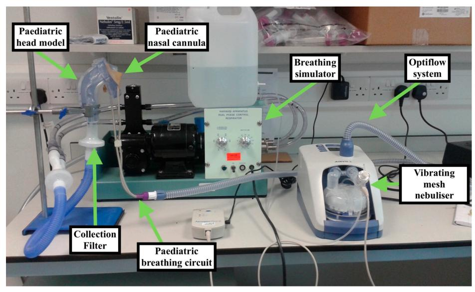
Figure S1. A photograph highlighting the physical setup for the paediatric nasal cannula set up.
