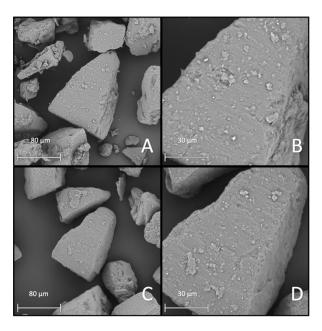
**Figure 6.** SEM images showing IH230HSM+. (**A**,**B**) Before and (**C**,**D**) after removing residual particles via air-jet sieving. (**A**,**C**) In  $1000 \times$  magnification and (**B**,**D**) in  $2500 \times$  magnification.
