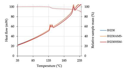
**Figure 2.** Results of DSC analysis of the raw material in comparison to processed powders without the additive. The secondary y-axis shows the relative mass decrease (dotted lines). n = 3. Negligible variation between the compared data series results in overlapping curves.
