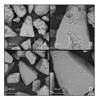
**Figure 5.** SEM images showing IH230AMS+. (**A**,**B**) Before and (**C**,**D**) after removing residual particles via air-jet sieving. (**A**,**C**) In  $1000 \times$  magnification and (**B**,**D**) in  $2500 \times$  magnification.
