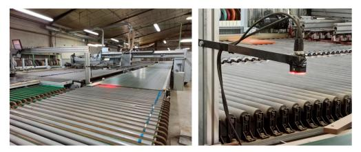
Figure 8. Camera scanning pieces in the conveyor of the edge banding machine.
