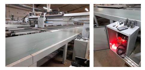
Figure 5. Edge banding machine and detail of the electrical cabinet in the production line.
