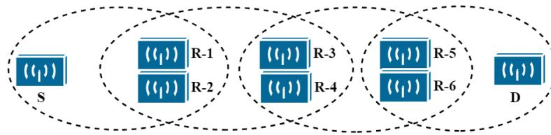
**Figure 6.** Network architecture of collocated relay nodes of a width of two with ideal coverage estimation.
