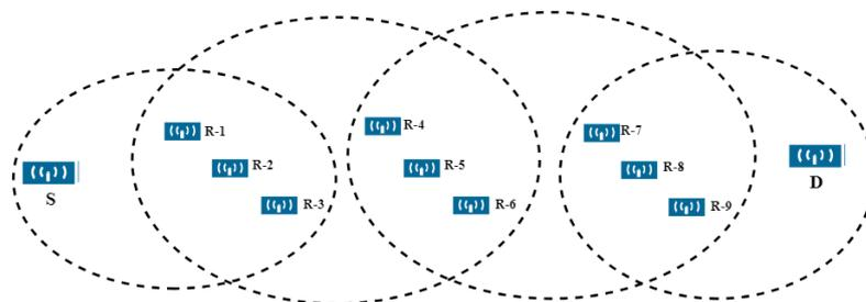
**Figure 9.** Network architecture of physically offset relay nodes of a width of three with ideal coverage estimation.
