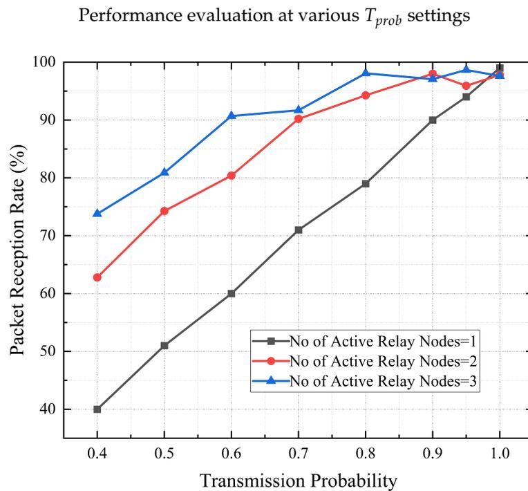
**Figure 13.** Performance comparison at various  $T_{prob}$  using the data from Tables 2 and 3.
