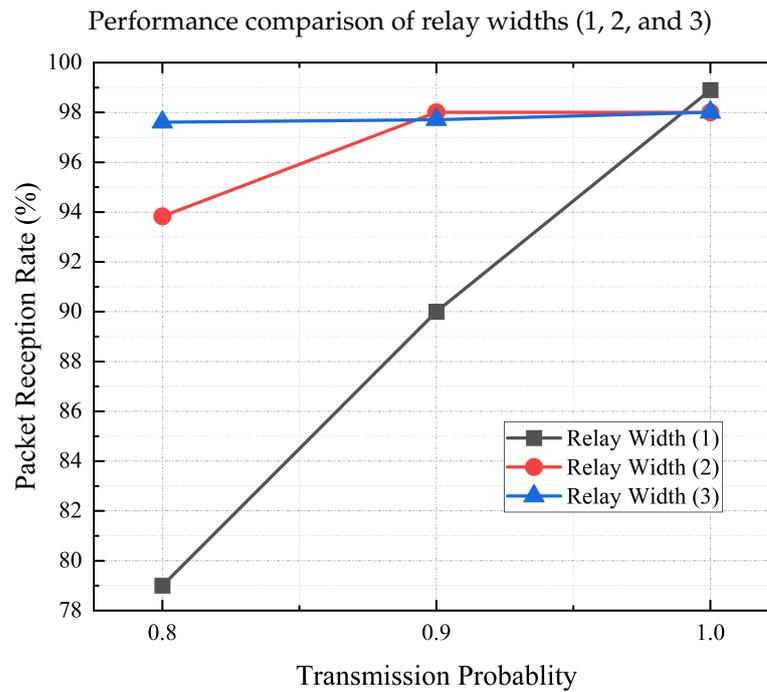
Figure 14. Performance comparison using a one-hop model.
