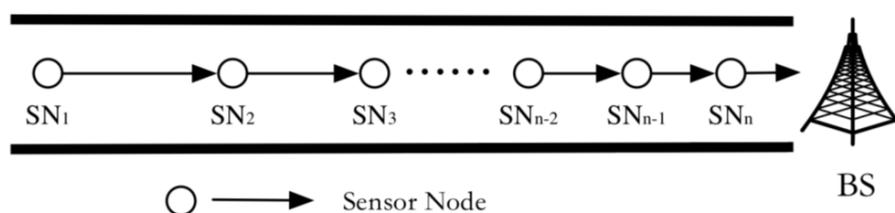
**Figure 2.** An example of a chain-type wireless sensor network [20].
