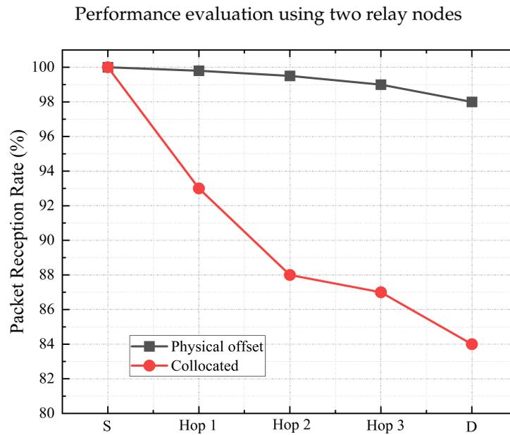
Figure 11. Overall performance using two relay nodes at each hop.
