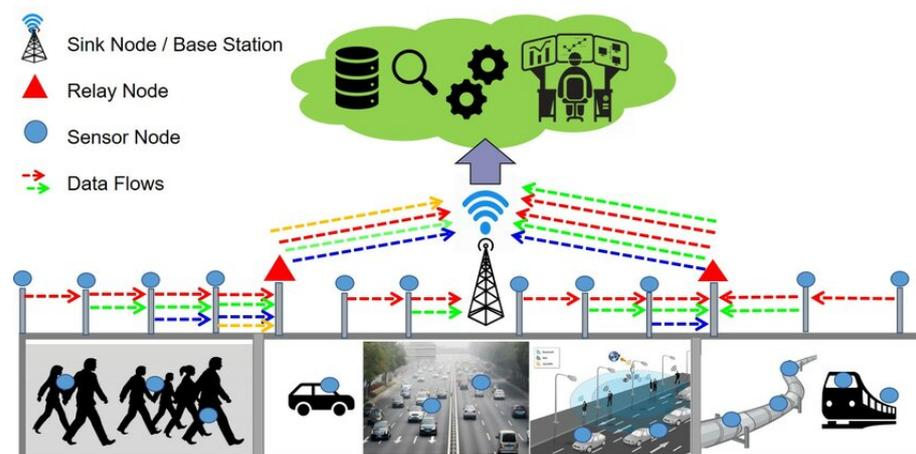
Figure 1. Linear wireless sensor networks and applications [13].
