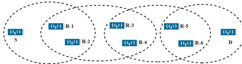
**Figure 7.** Network architecture of physically offset relay nodes of a width of two with ideal coverage estimation.
