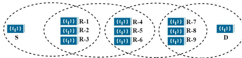
**Figure 8.** Network architecture of collocated relay nodes of a width of three with ideal coverage estimation.
