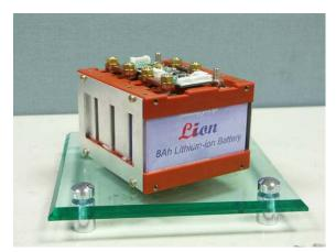
Fig. 5 Appearance of 14.4V Lithium-ion battery module
