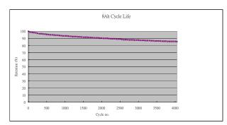
Fig. 4 Cycle life characteristic of 8Ah Lithium-ion cell (charge and discharge at 60%-80% SOC)
