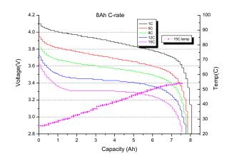
Fig. 2 Different C-rate discharge capability of 8Ah Lithium-ion cell (cell charged with 1C rate at all test condition)
