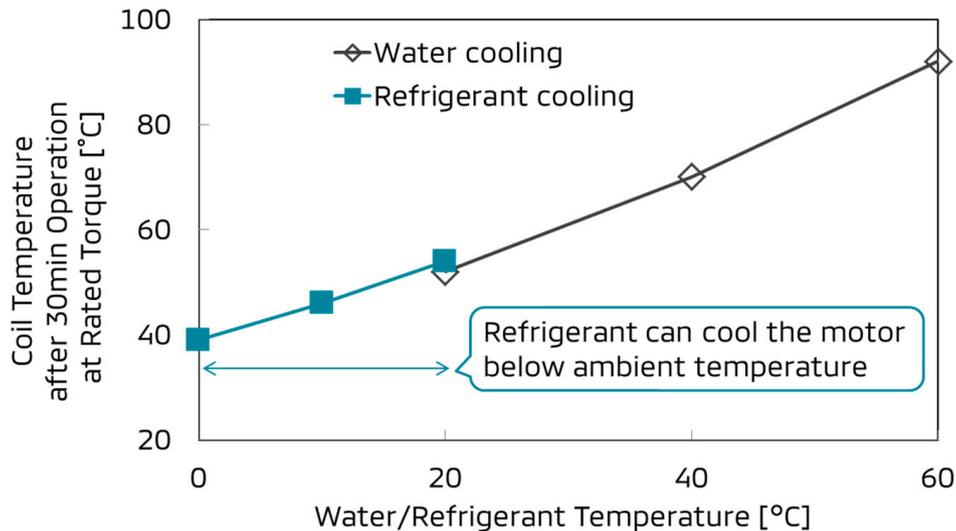
**Figure 6.** Coil temperature after 30 min operation at rated torque vs water temperature or refrigerant temperature.
