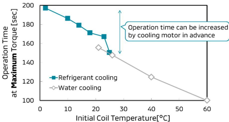
**Figure 11.** Operation time at maximum torque vs initial coil temperature.
