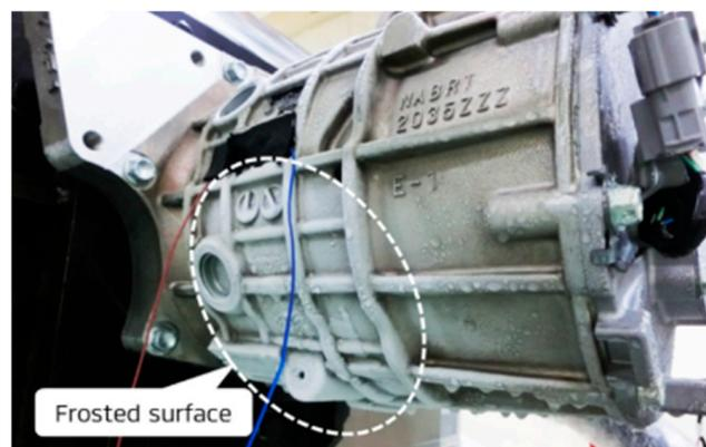
**Figure 7.** Frosted motor surface by refrigerant cooling.
