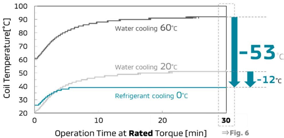
Figure 5. Operation time at rated torque vs coil temperature.
