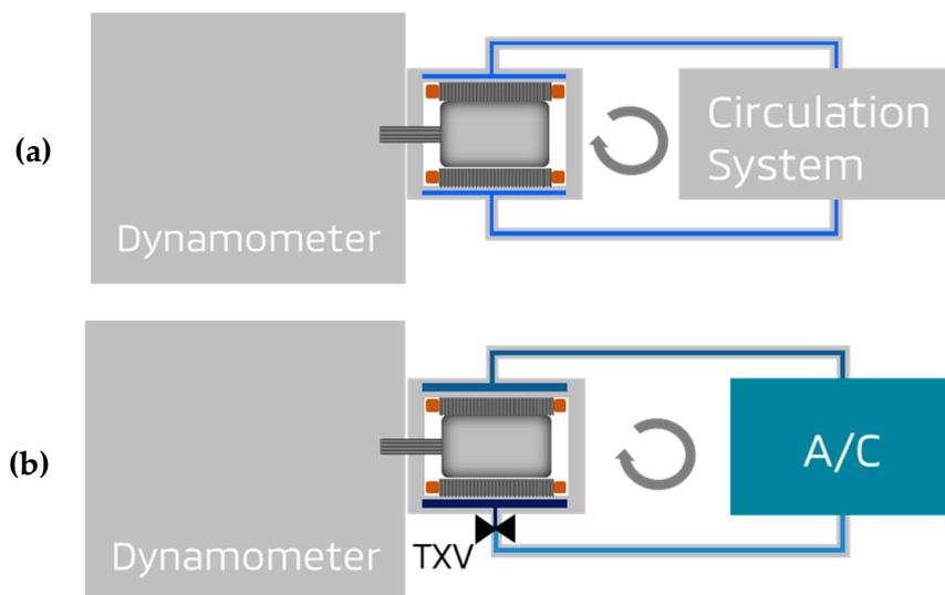
Figure 4. Experimental setup: (a) Water cooling; (b) refrigerant cooling.
