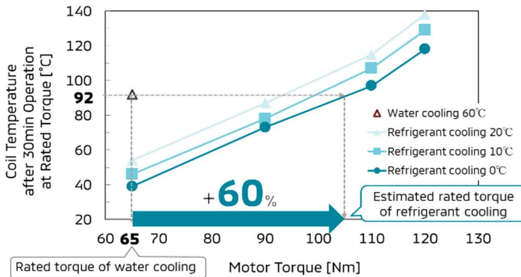
Figure 8. Coil temperature after 30 min operation vs motor torque.
