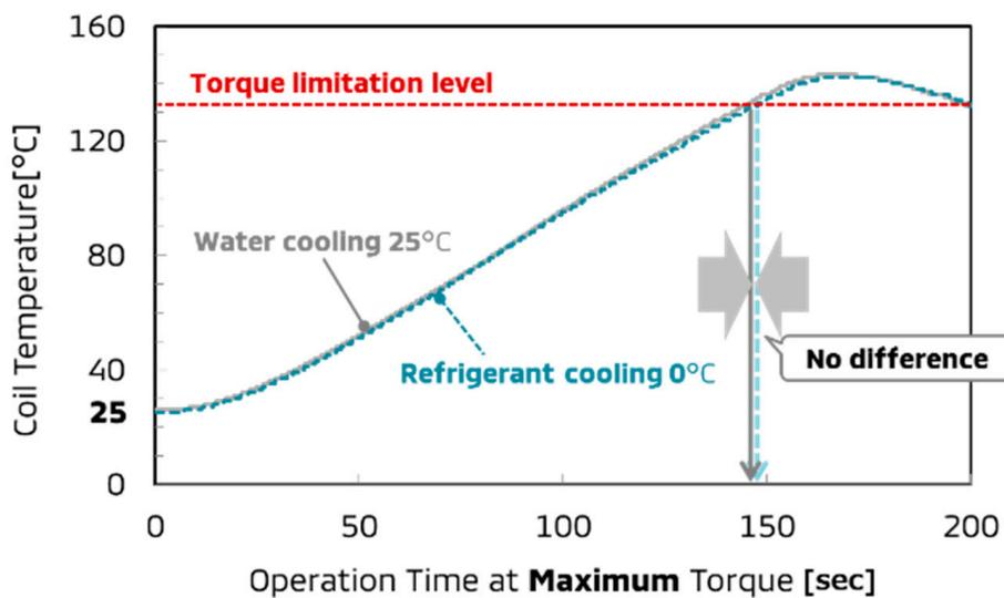
Figure 9. Coil temperature vs operation time at maximum torque.
