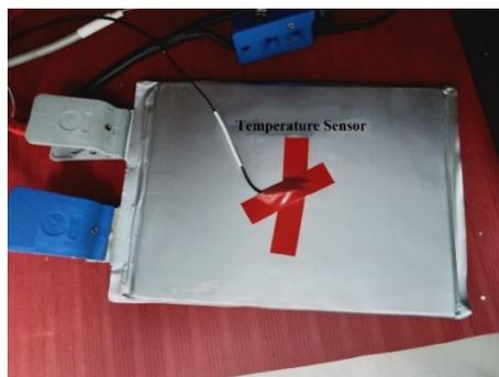
**Figure 5.** 30 Ah pouch LiFePO<sub>4</sub> lithium-ion battery.
