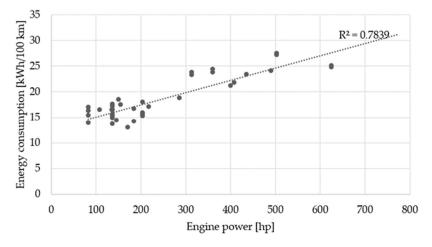
Figure A3. The relationship between engine power [hp] and energy consumption [kWh/100 km].
