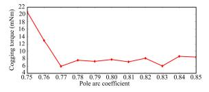
**Figure 8.** Effect of pole arc coefficient on cogging torque in a machine with a 4-pole and 33-slot combination.
