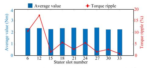
**Figure 5.** The average value and torque ripple of electromagnetic torque under different numbers of stator slots when the number of rotor poles is 4.
