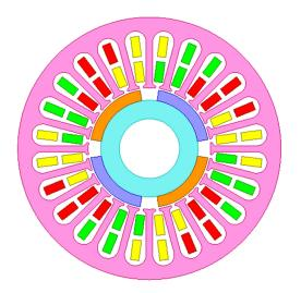
Figure 1. Structure diagram of a 4-pole and 24-slot surface-mounted permanent magnet (SPM) machine.
