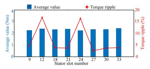
**Figure 6.** The average value and torque ripple of electromagnetic torque under different numbers of stator slots when the number of rotor poles is 8.
