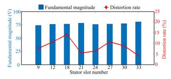
**Figure 3.** The variation in back EMF with the variation in the number of stator slots when the number of rotor poles is 8.
