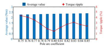
**Figure 13.** Effect of pole arc coefficient on electromagnetic torque in a machine with 10-pole and 21-slot.
