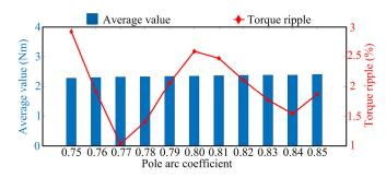
**Figure 12.** Effect of pole arc coefficient on electromagnetic torque in a machine with 8-pole and 27-slot.
