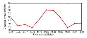
**Figure 9.** Effect of pole arc coefficient on cogging torque in a machine with an 8-pole and 27-slot combination.
