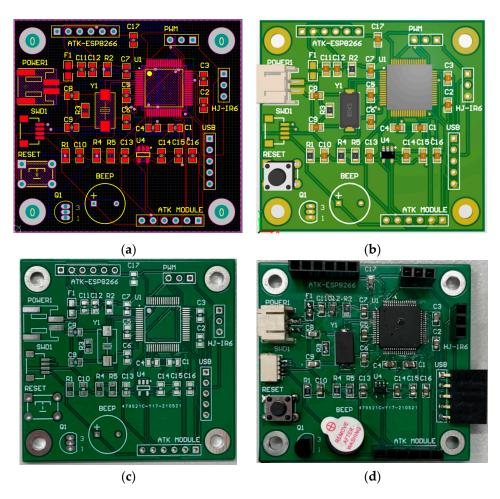
**Figure 5.** Preview and physical view of the control board: (a) preview of the layout wiring; (b) preview of the PCB; (c) physical view of the control board before welding; (d) physical view of the control board after welding.
