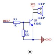
Figure 4. Circuit schematic: (a) chip; (b) reset circuit; (c) start-up model; (d) power filter circuit; (e) crystal resonance circuit; (f) voltage conversion circuit; (g) current foldback circuit; (h) power supply; (i) SWD external interface; (j) USB external interface; (k) MPU6050 external interface; (l) ATK-ESP8266 WIFI; (m) PWM external interface and interface of speed measuring module; (n) buzzer alarm circuit.
