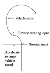
Figure 6. Schematic diagram of layout path of fishhook testing ground.
