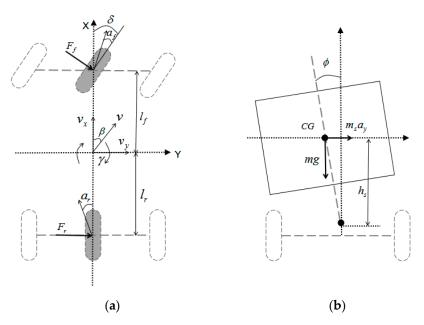
Figure 1. Three-degree-of-freedom cartwheel dynamics model: (a) top view; (b) rear view.
