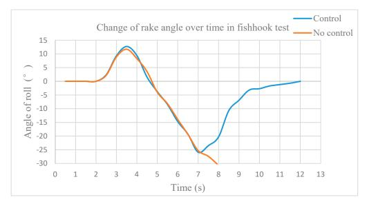
Figure 8. Change of rake angle over time in fishhook test.
