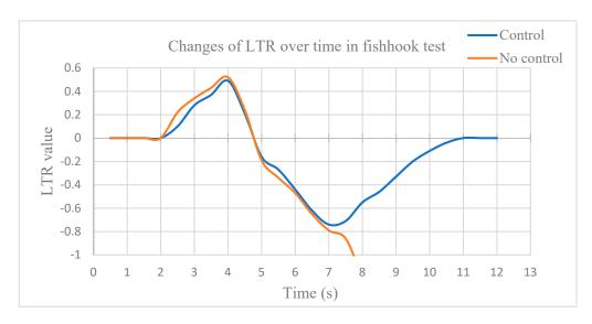
Figure 10. Changes of LTR over time in fishhook test.
