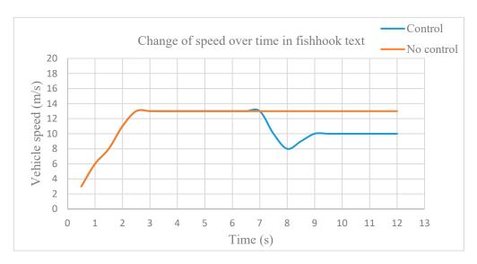
Figure 9. Change of speed over time in fishhook text.
