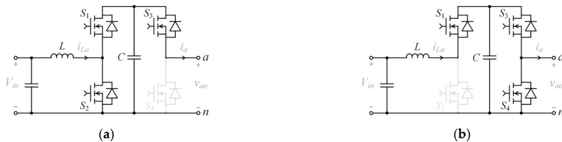
**Figure 2.** The two modes of a phase module of the BBI: (a) boost mode and (b) buck mode.
