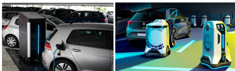
Figure 2. Mobile charging stations from Mob-Energy [10] and Volkswagen [11].
