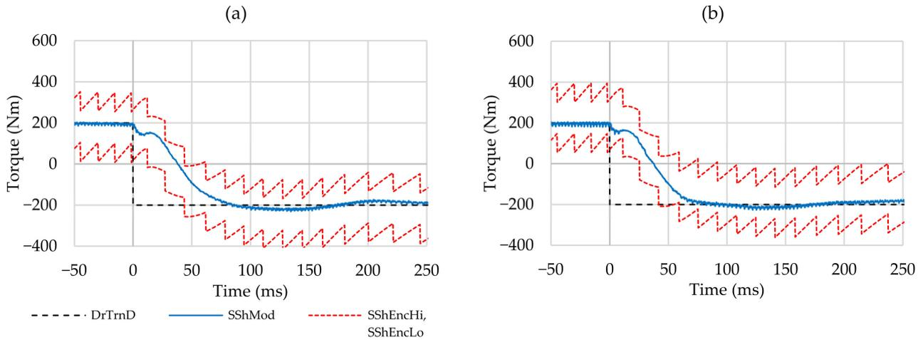
**Figure 13.** Measurements for a dynamic change from driving to regenerative braking by a step change in desired drivetrain torque  $M_{DrTrnD}$  from 200 Nm to  $-200$  Nm shortly after driving off in the case of the earliest possible (a) and the latest possible (b) first edge.
