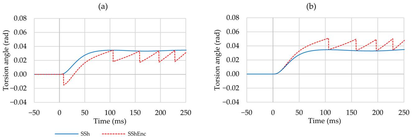
**Figure 6.** Torsion angle of the side shaft during driving-off from standstill in the case of the earliest possible (a) and the latest possible (b) first edge.
