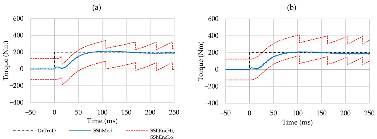
**Figure 9.** Measurements of a driving-off procedure with the driver's desired torque of 200 Nm in the case of the earliest possible (a) and the latest possible (b) first edge.
