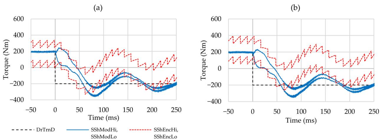
**Figure 16.** Measurements of both bands for a fault event for a dynamic change from driving to regenerative braking by a step change in desired drivetrain torque  $M_{DrTrnD}$  from 200 Nm to  $-200$  Nm shortly after driving off in the case of the earliest possible (a) and the latest possible (b) first edge.
