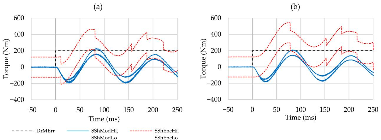
**Figure 17.** Measurements of both bands for a fault event at standstill with a step change in torque  $M_{DrMErr}$  from 0 Nm to 200 Nm in the case of the earliest possible (a) and the latest possible (b) first edge.
