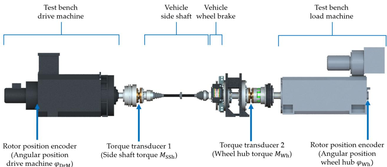
**Figure 1.** Positions of the relevant sensors of the applied HiL test bench and the corresponding measured values.
