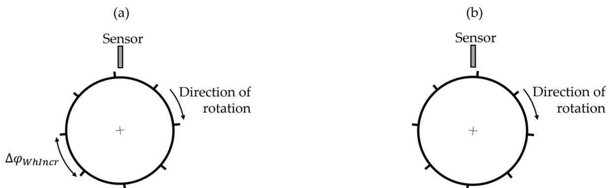
**Figure 5.** Initial positions of the vehicle wheel hub at vehicle standstill with an early (a) and a late (b) first edge.
