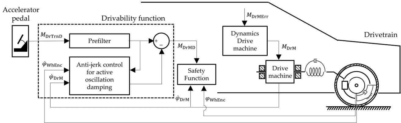
Figure 11. Overview of the considered system in the case of a drive machine error.
