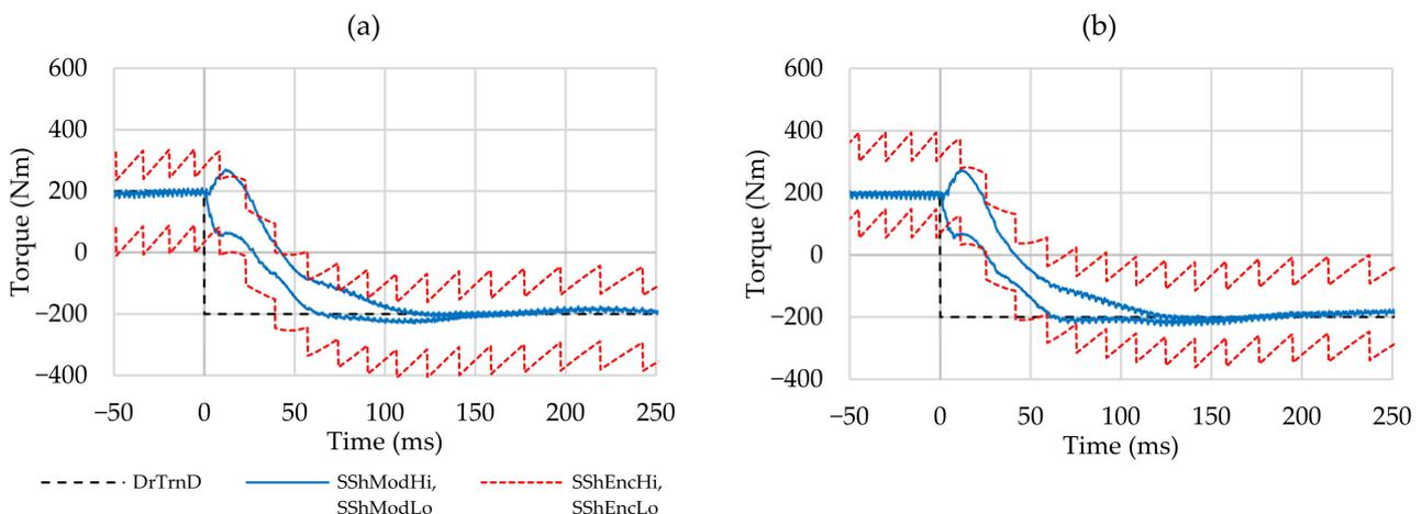
Figure 15. Measurements of both bands for a dynamic change from driving to regenerative braking by a step change in desired drivetrain torque  $M_{DrTrmD}$  from 200 Nm to  $-200$  Nm shortly after driving off in the case of the earliest possible (a) and the latest possible (b) first edge.
