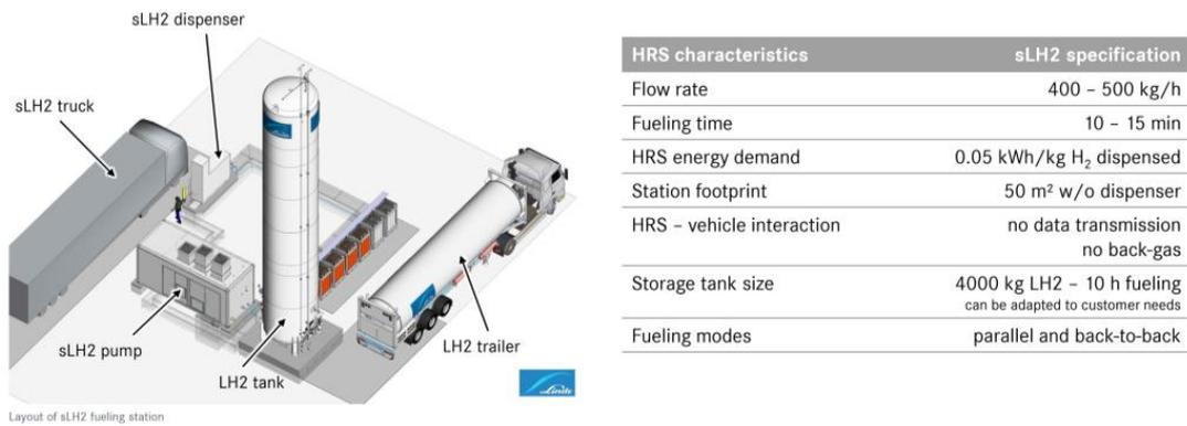
Figure 4. Exemplary layout of a small sLH2 HRS with one dispenser.
