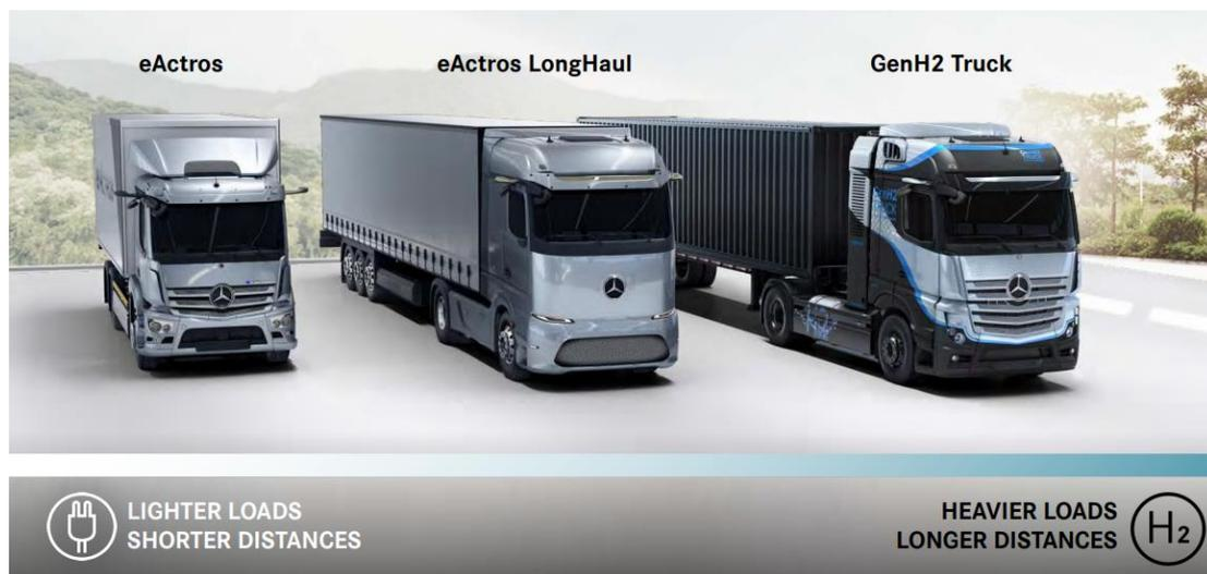
**Figure 1.** Technology fit for commercial vehicles based on different use requirements: battery electric trucks, eActros (left) and eActros LongHaul (middle), and the GenH2 truck using liquid hydrogen in a fuel cell (right) (source: Daimler Truck Capital Market Day—November, 2021).
