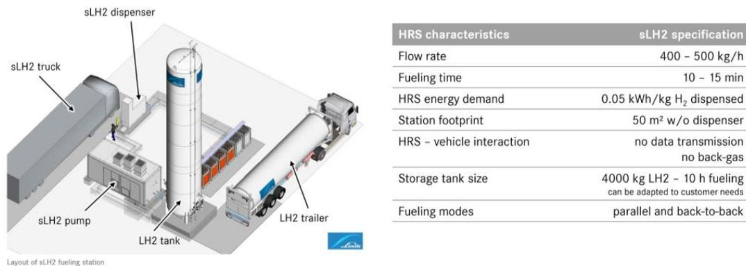
**Figure 4.** Exemplary layout of a small sLH<sub>2</sub> HRS with one dispenser.
