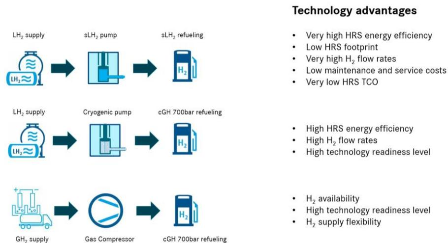
**Figure 5.** Technology advantages of different fueling technologies (sLH<sub>2</sub> on top).
