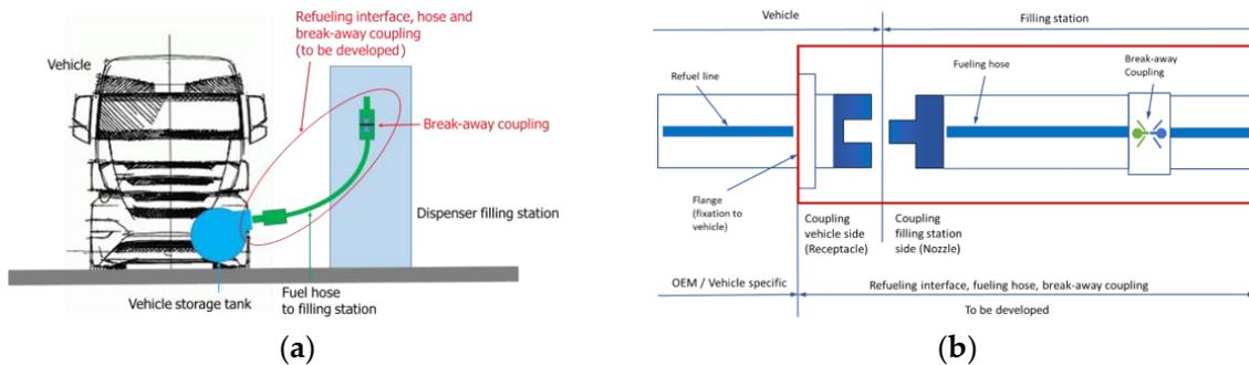
Figure 7. (a) Overview of the fueling interface-components; (b) Overview of system boundaries and interface with focus of standardization effort highlighted in red box.
