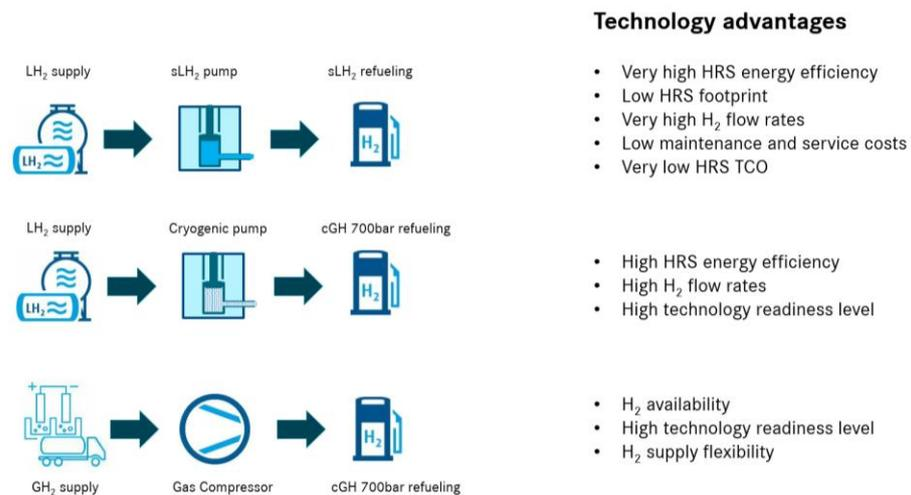
Figure 5. Technology advantages of different fueling technologies (sLH2 on top).
