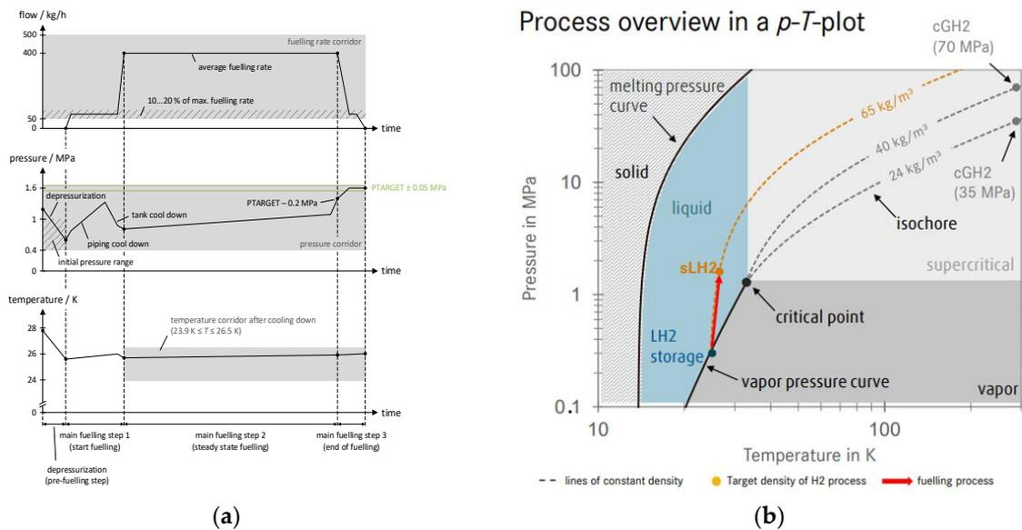
Figure 6. (a) Exemplarily flow, pressure and temperature profiles during sLH2 fueling; (b) p–T plot of hydrogen sLH2.
