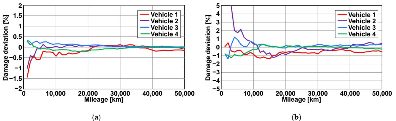
**Figure 9.** Damage deviation of the rollover classification. (a) Damage deviation of the rollover classification with 10 Hz data; (b) damage deviation of the rollover classification with 1 Hz data.
