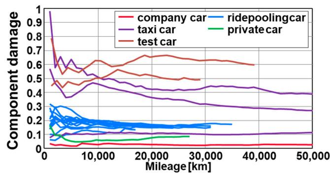
Figure 18. Component damages in relation to the data size.
