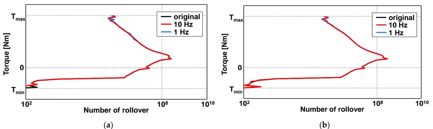
Figure 8. Exemplary results of the rollover classification. (a) Rollover classification for the data of 10,000 km; (b) rollover classification for the data of 50,000 km.
