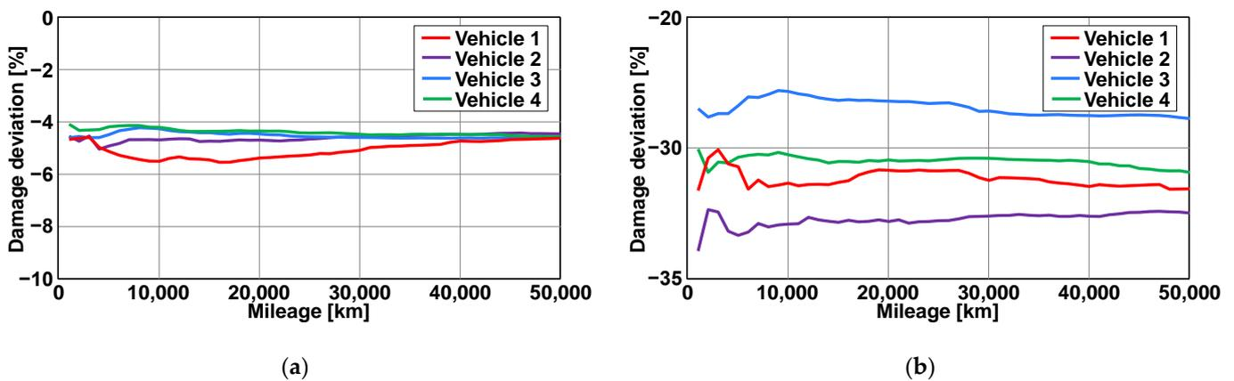
Figure 15. Damage deviation of the EM torque rainflow classification. (a) Damage deviation of the EM torque rainflow classification with 10 Hz data; (b) damage deviation of the EM torque rainflow classification with 1 Hz data.
