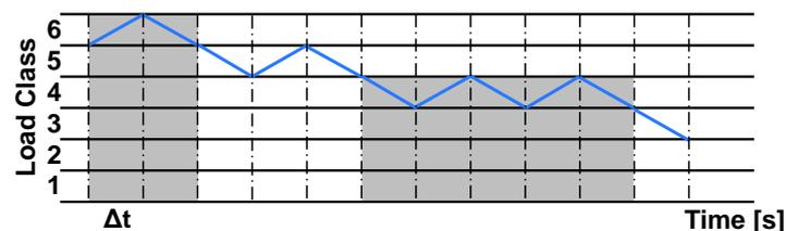
Figure 3. Time at level classification with defined load classes from 1 to 6 and the time interval  $\Delta t$ .
