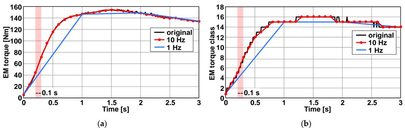
**Figure 6.** EM torque for 3 s from the selected data. (a) The original torque and the torque after downsampling; (b) classified EM torques at different frequencies with 10 Nm as the class width.
