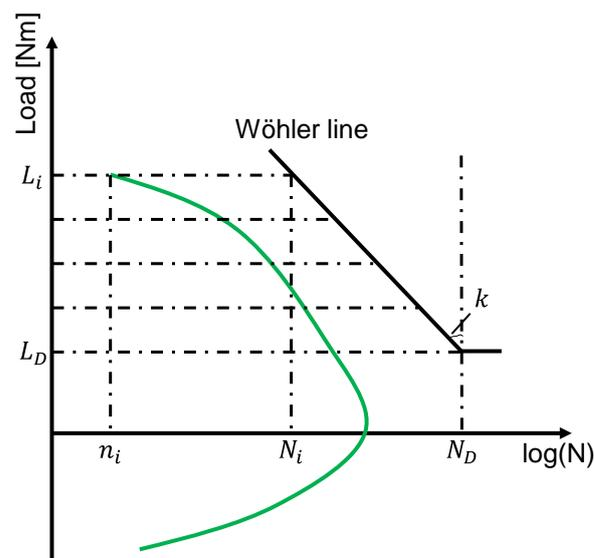
Figure 1. Wöhler line for the lifetime calculation with torque as the load.
