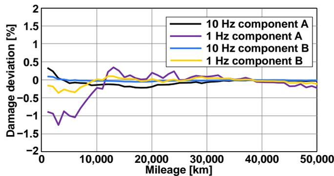
Figure 11. Impact of the Wöhler line on the damage deviation of the rollover classification.
