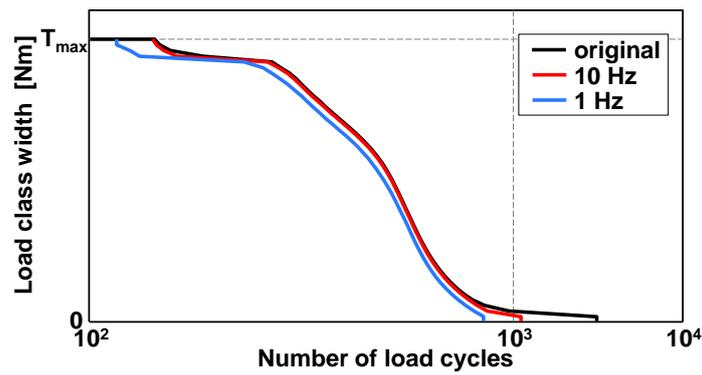
Figure 14. Rainflow classification for torque with 10,000 km data in the range pair format.
