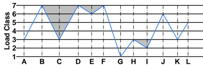
Figure 4. Rainflow classification with defined torque classes from 1 to 7 and load extremes from A to L.
