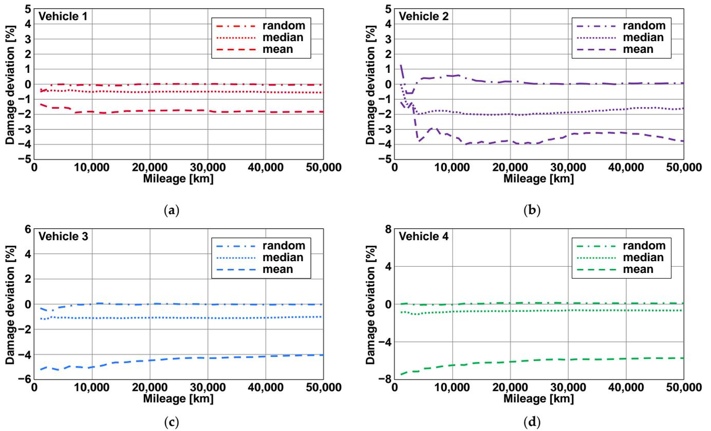
Figure 10. Damage deviation of the rollover classification after signal preprocessing. (a) Vehicle 1; (b) vehicle 2; (c) vehicle 3; (d) vehicle 4.
