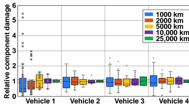
Figure 17. Damage variability of the data with different data sizes.
