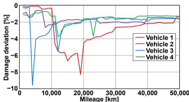
Figure 16. Damage deviation of the temperature rainflow classification.
