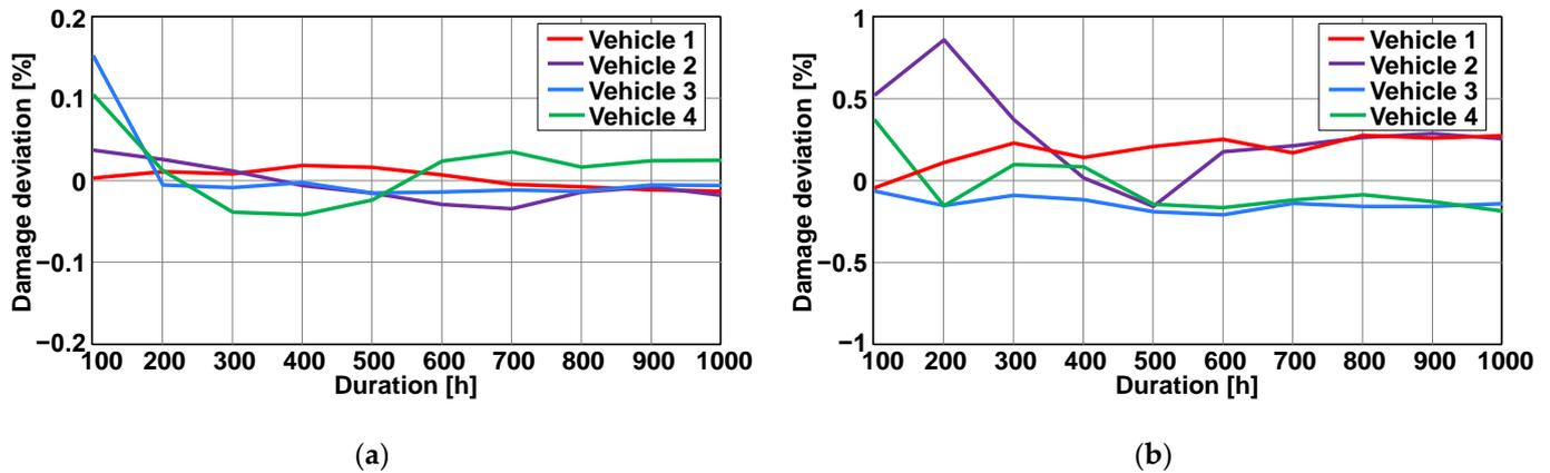
**Figure 12.** Damage deviation of the time at level classification for EM power. (a) Damage deviation of the time at level classification for EM power with 10 Hz data; (b) damage deviation of the time at level classification for EM power with 1 Hz data.
