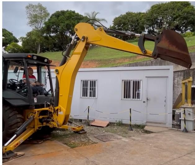
**Figure 14.** Trenching experimental test performed with the hybrid backhoe loader.
