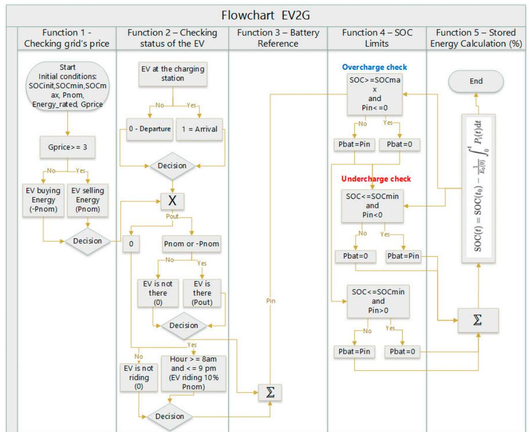
**Figure 2.** A sketch of a logic diagram of the reference to EV2G, providing an overview of the model for both charging and discharging.
